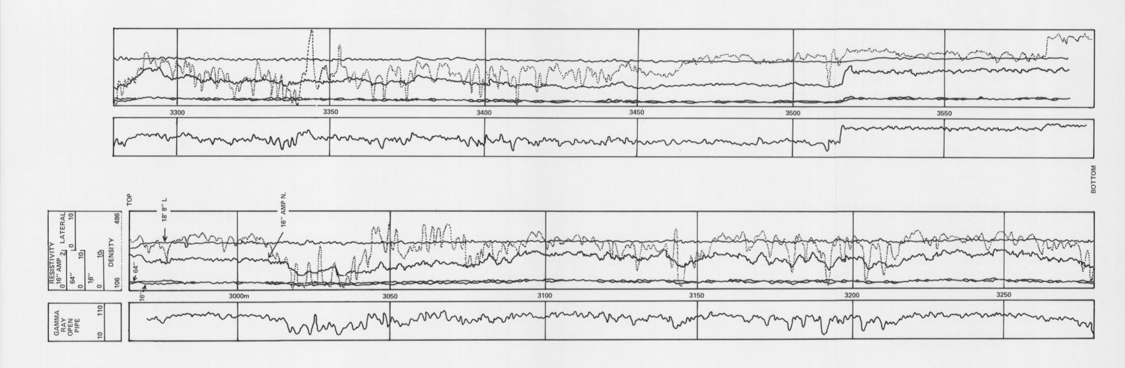
Figure 3 Composite electric log, gamma gamma density log and natural gamma radiation log for Hole 1.
