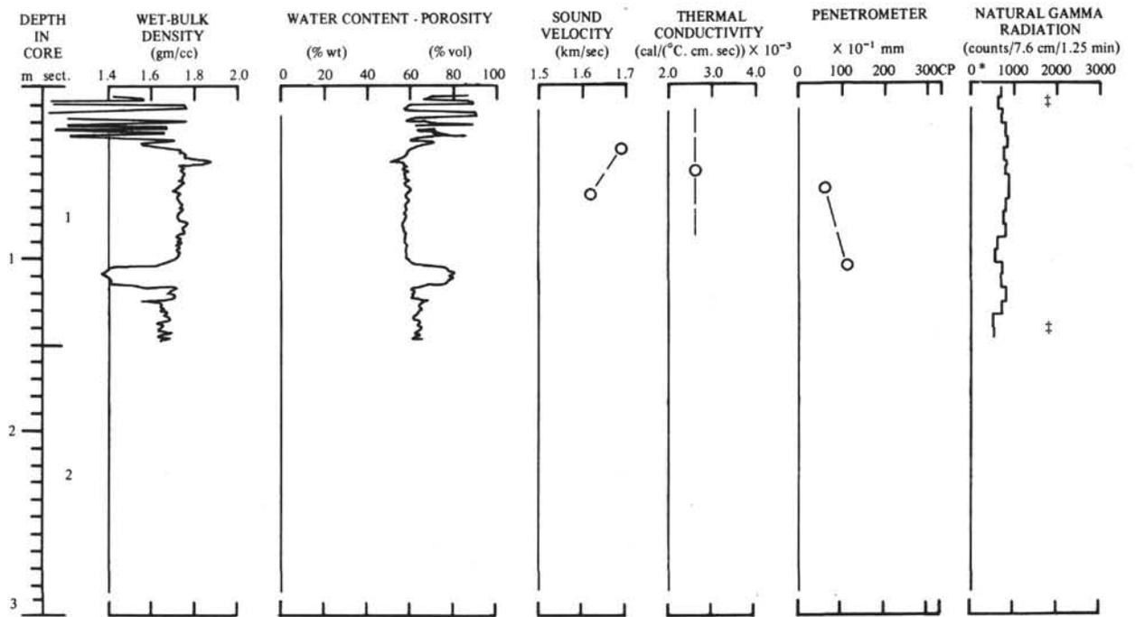
Figure 11A. *Physical Properties of Core 4, Hole 13A.*
