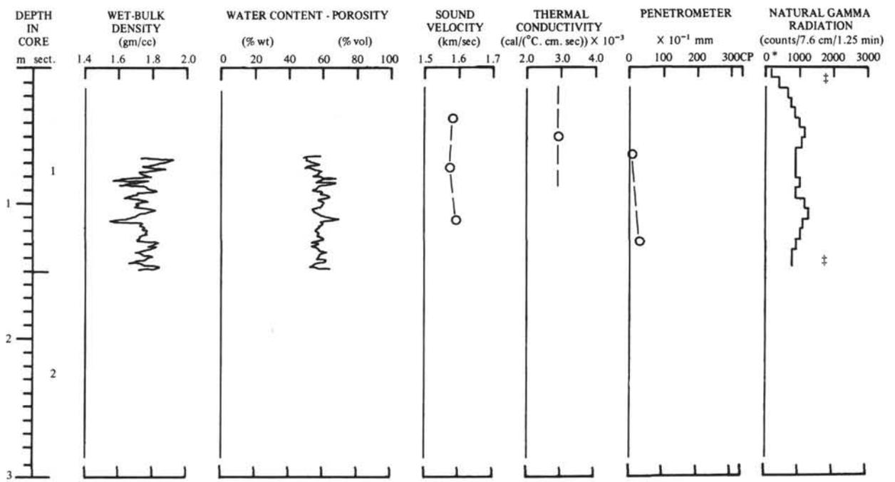
Figure 12A. *Physical properties of Core 5, Hole 13A.*
