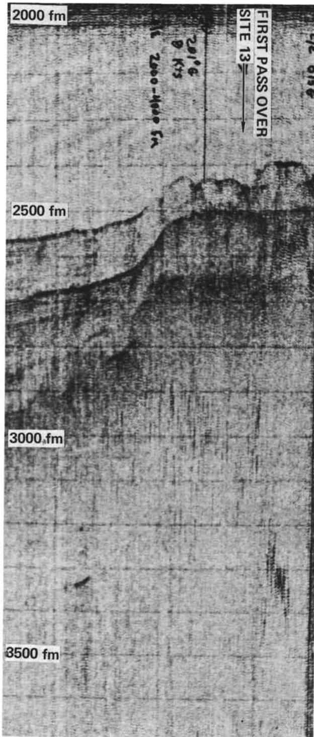
Figure 1. Continuous seismic profiler record in the vicinity of Site 13.
