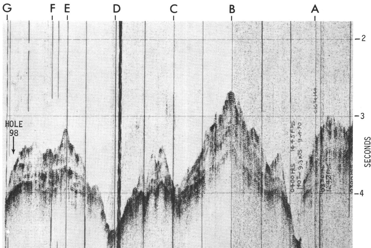
Figure 2a. Glomar Challenger seismic record near Site 98. See Figure 1 for track location.
