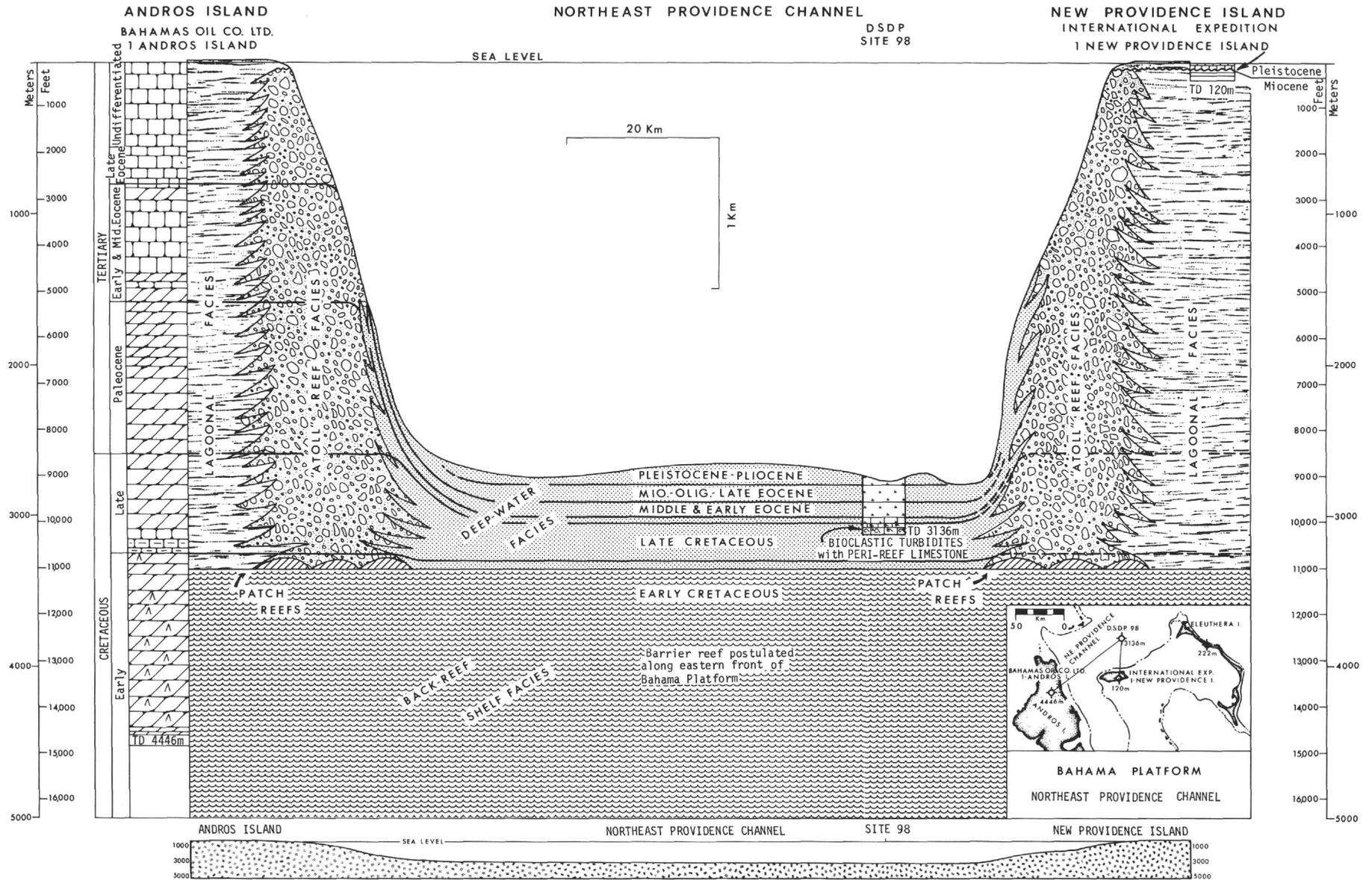
Figure 6. Cross-section of a portion of the Bahama Platform through Site 98 from Andros Island to New Providence Island showing the relationships of shallow-water bank and shelf facies to the deep-water channel facies. Time lines are based on ages from the Andros Island well and the Site 98 core hole.
