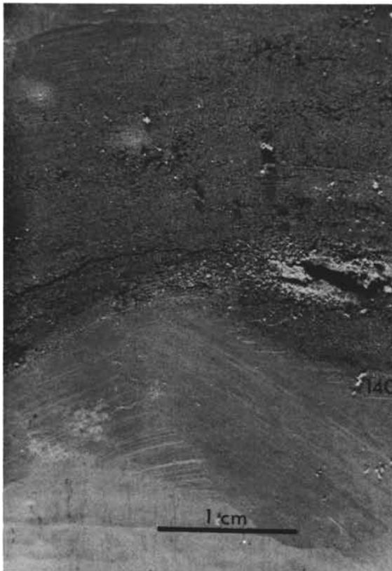
Figure 9. Illustration of a graded sand interval at the base of a terrigenous mud layer in Section 2, Core 2 of Hole 130. Such basal layers are usually poorly sorted and occasionally finely laminated. Some evidence of scour or winnowing at the basal contact is seen. For example, the pocket of sand seen just above the 140 cm marking is perhaps the filling of a groove or flute depression.
