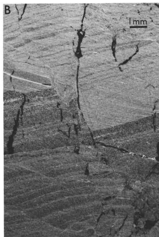
Figure 4. Reverse prints of thin-sections of samples from the Mistral-1 well in the Gulf of Lyon. (A) a metagraywacke from Core 2. Note the extreme similarity of this specimen with Sample 134-D-3-CC in Figure 2 (C). (B) a laminated phyllite from Core 3, which except for fracturing and shearing is comparable to Sample 134-B-1-CC in Figure 28.
