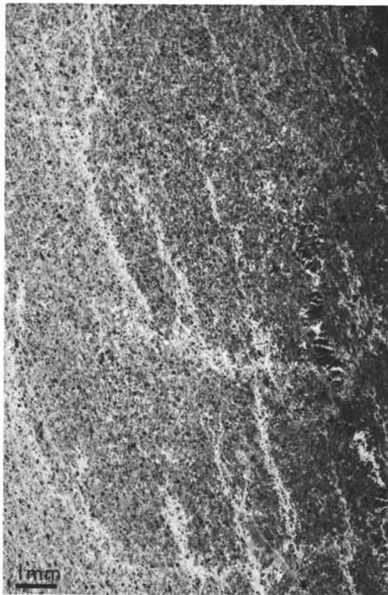
Figure 1. Reverse print of a thin-section microphotograph of Sample 13-133-3-CC from the western Sardinia Slope. Note the orientation of the metamorphic fabric parallel to the elongation of quartz grains (black), and the quartz filled veins.
