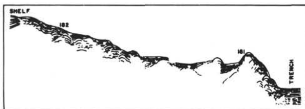
Figure 1. Diagrammatic section across the continental slope (after seismic reflection records) showing setting of Sites 181 and 182.
