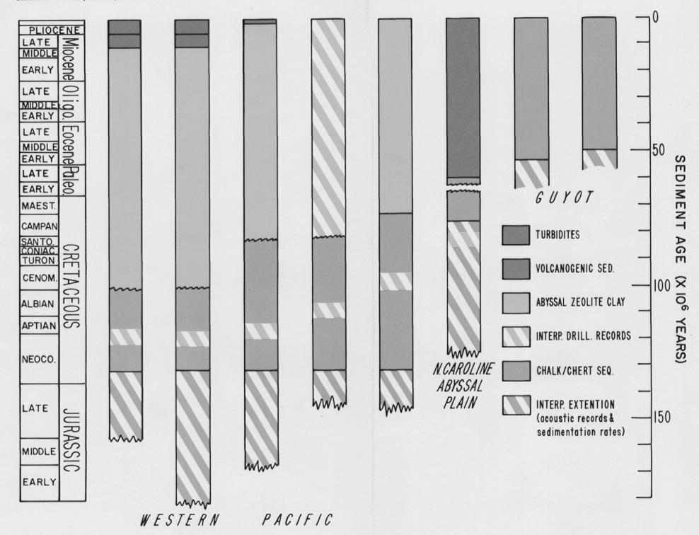
Figure 1. Summary of Leg 20 drilling results. Vertical columns indicate lithology vs. age for each site. Extrapolations beyond total depth based on an interpretation of seismic reflection profiles obtained at each site.
