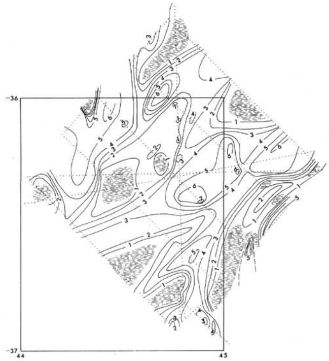
Figure 3. Sediment isopach map of the survey area. Contour interval tenth of a second (two-way travel time). Basement outcrops are shown by hachures.
