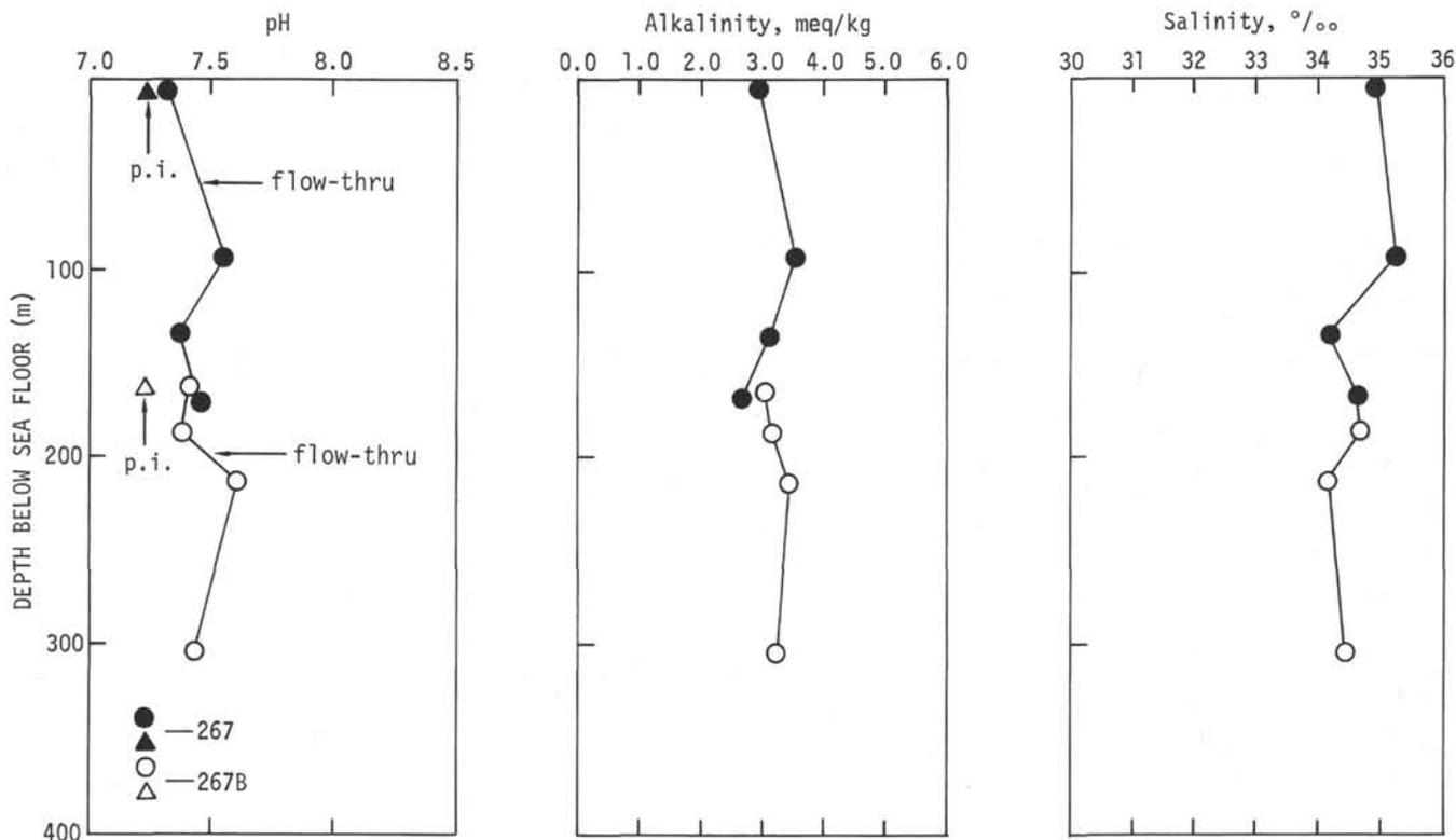
Figure 5. Shipboard measurements of pH, alkalinity, and salinity of sediment pore waters at Site 267.
