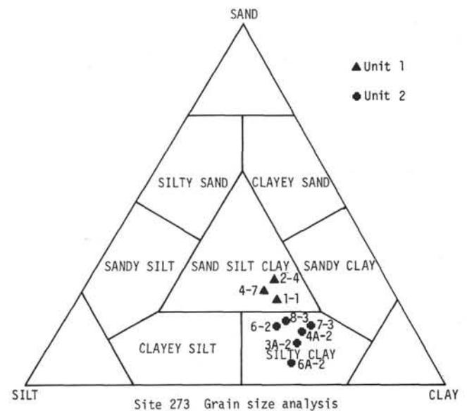
Figure 3. Grain size analyses from lithologic Units 1 and 2 at Site 273. Numbers next to symbols refer to core and section.
