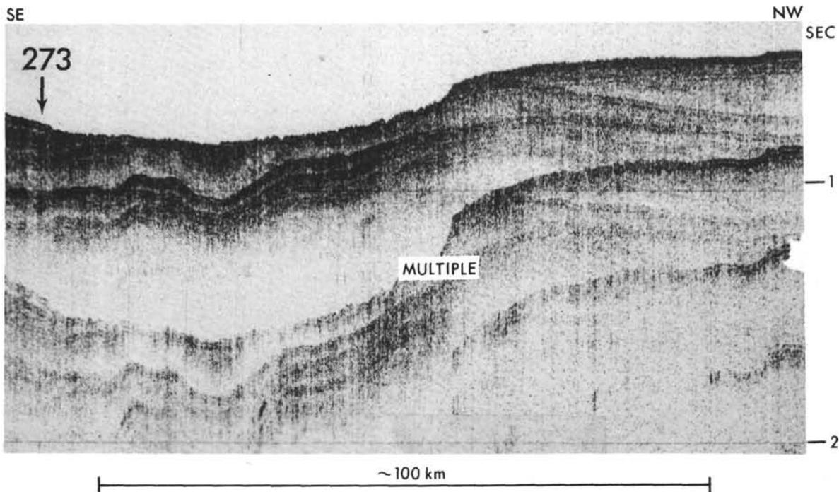
Figure 2. Glomar Challenger acoustic reflection profile on approach to Site 273. Vertical scale is in seconds of two-way reflection time. Location of profile shown in Figure 1.
