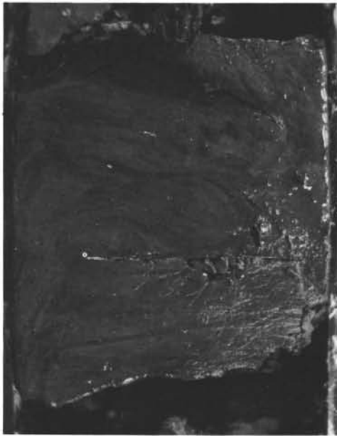
Figure 2. Indurated mudstone reconstituted from sediment slurry under bit weight. This mudstone was cut with the band saw, lifted out of the core liner, and washed clean under running water. Sample 28-274-43-4.
