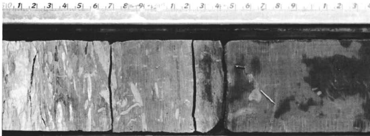
Figure 15. Bioturbated nanno limestone in contact with uppermost vitric tuff (also bioturbated). Contact falls at 63 cm. Uppermost tuff contains 30 m.y. hiatus between Albian to mid-Campanian. 289-131-1, Unit 2B, Site 289.
