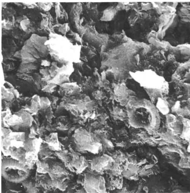
Figure 5. SEM photograph. Site 287; hole depth, 236.6 meters; Unit 5, semilithified nanno-chalk; solution very strong, encrusting cristobalite common, strong grain cementation; \times 2260 .
