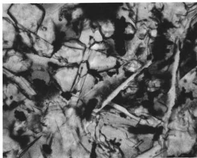
Figure 8. 332A-8-1, #13c. Gray areas with the skeletal magnetite grains were glass that has been replaced by smectite. Some of the areas show fibers and minute dark brown spots typical of the glass phase. Bar scale is 0.02 mm long. Plane light.
