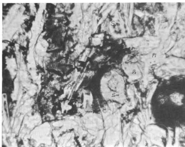
Figure 1. 332A-7-2, #18. Round globules of smectite in dark magnetite and fiber-filled glass. G1-glass; P1-plagioclase; Px-pyroxene; Sm-smectite. Bar scale is 0.02 mm long. Plane light.
