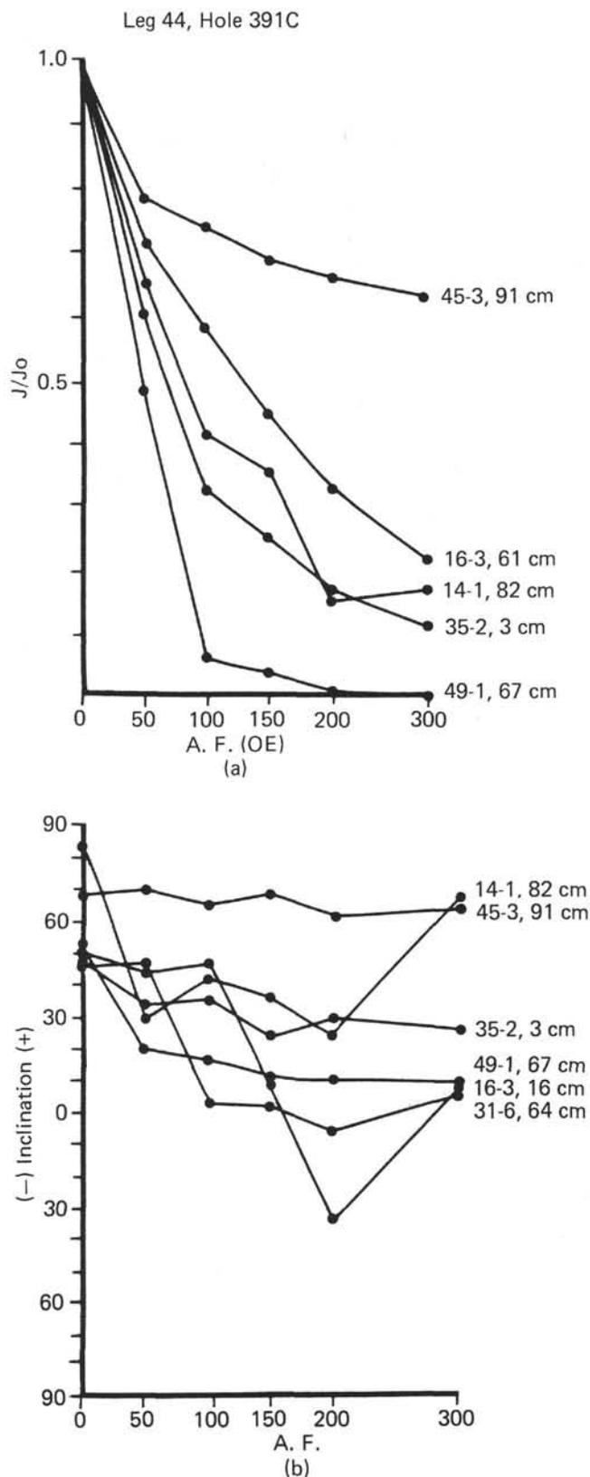
Figure 1. (a) Demagnetization curve showing the change in intensity on demagnetization for "pilot study" samples; and (b) Plot of change in inclination on demagnetization for "pilot study" samples.
