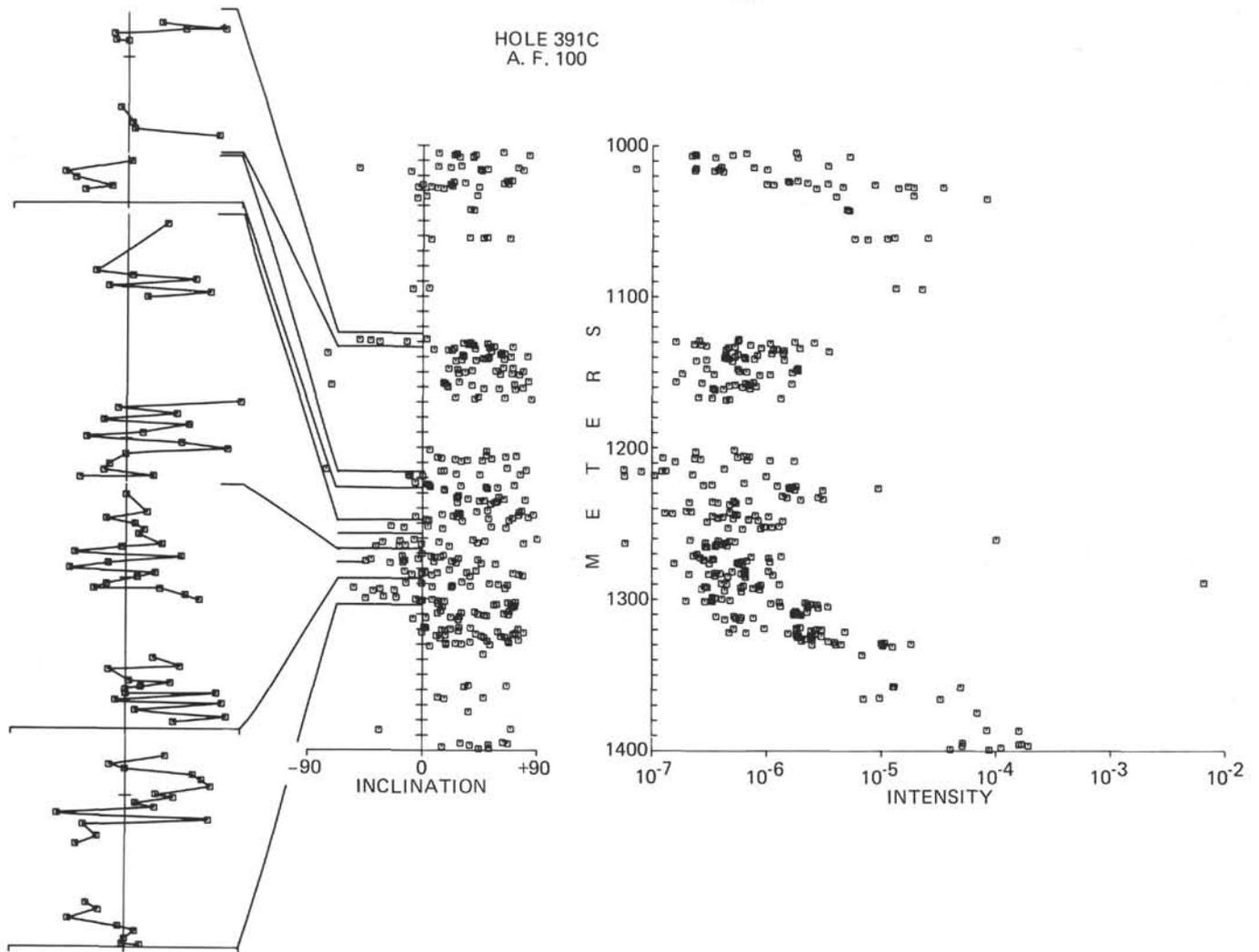
Figure 3. Plot of demagnetized sample inclinations and intensities against depth. Depths on vertical scale are from the drill rig floor. Reversed polarity intervals have been plotted at an enlarged vertical scale and are shown at left.
