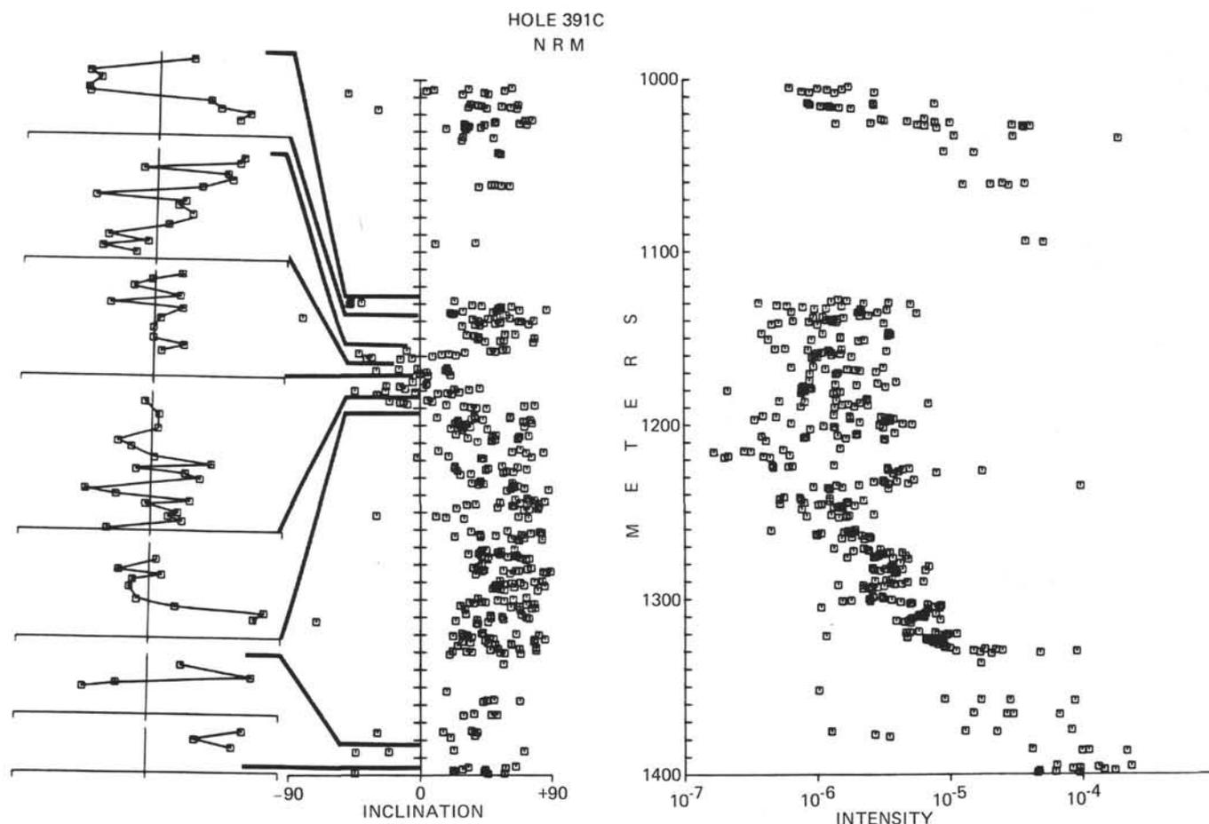
Figure 2. Plot of sample NRM inclinations and intensities against depth for samples from DSDP Hole 391C. Sample intensity is measured in emu. Depths are from the drill rig floor. Gaps between data points are a result of poor recovery. The vertical scale for intervals of reversed polarity has been expanded by a factor of 10 and the expanded data points are shown to the left of the diagram.
