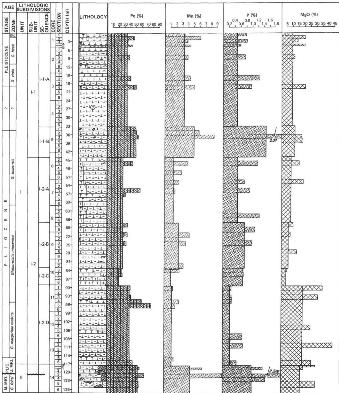
Figure 4. Distribution of Fe, Mn, P, and MgO (wt. %, recalculated to M. B.) in the section of upper Cenozoic sediments, region of the Mid-Atlantic Ridge, Hole 396, Leg 45.
