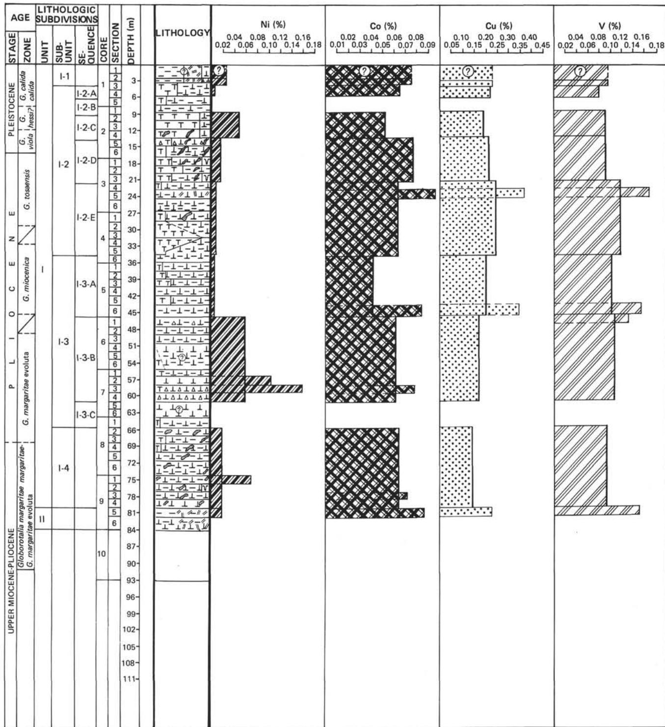
Figure 2. Distribution of Ni, Co, Cu, V (wt. %, recalculated to M.B.) in the section of upper Cenozoic sediments, region of the Mid-Atlantic Ridge, Hole 395, Leg 45.
