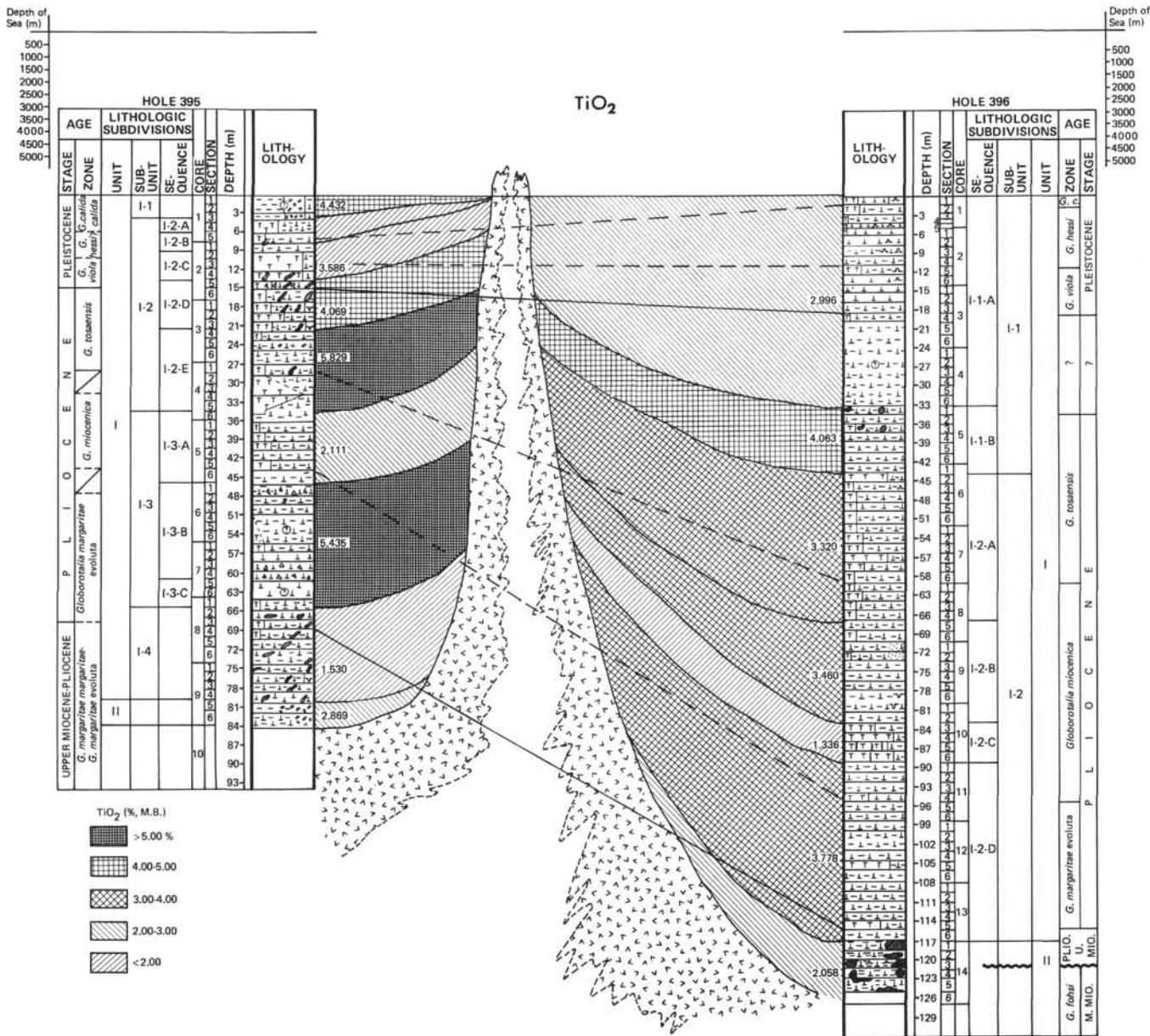
Figure 14. Schematic profile of  $\text{TiO}_2$  distribution in upper Cenozoic sediments, region of the Mid-Atlantic Ridge, Leg 45 (wt. %, M.B.).
