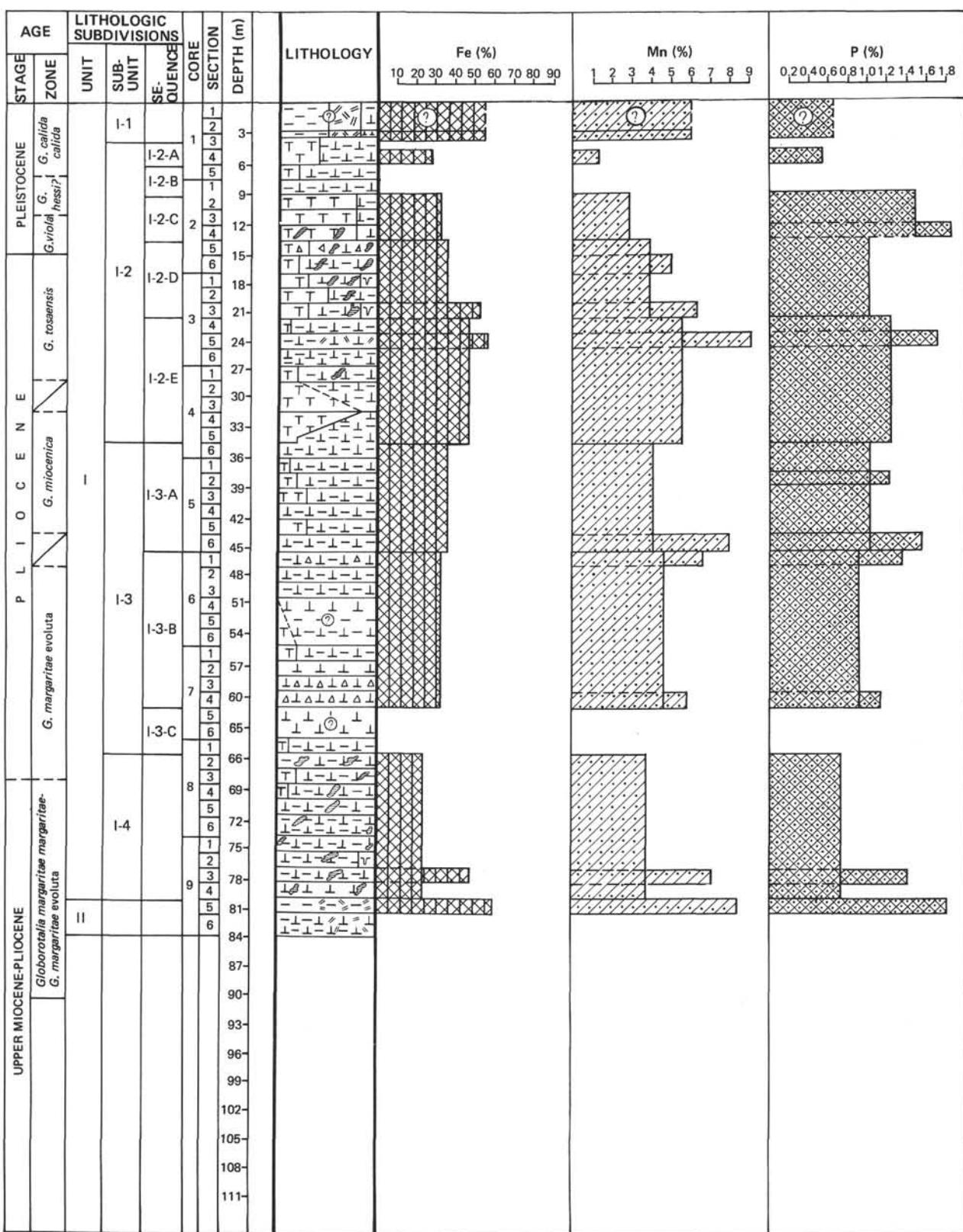
Figure 1. Distribution of Fe, Mn, P (wt. %, recalculated to the clastic-free, carbonate-free basis (M. B.)) in the section of upper Cenozoic sediments, region of the Mid-Atlantic Ridge, Hole 395, Leg 45.
