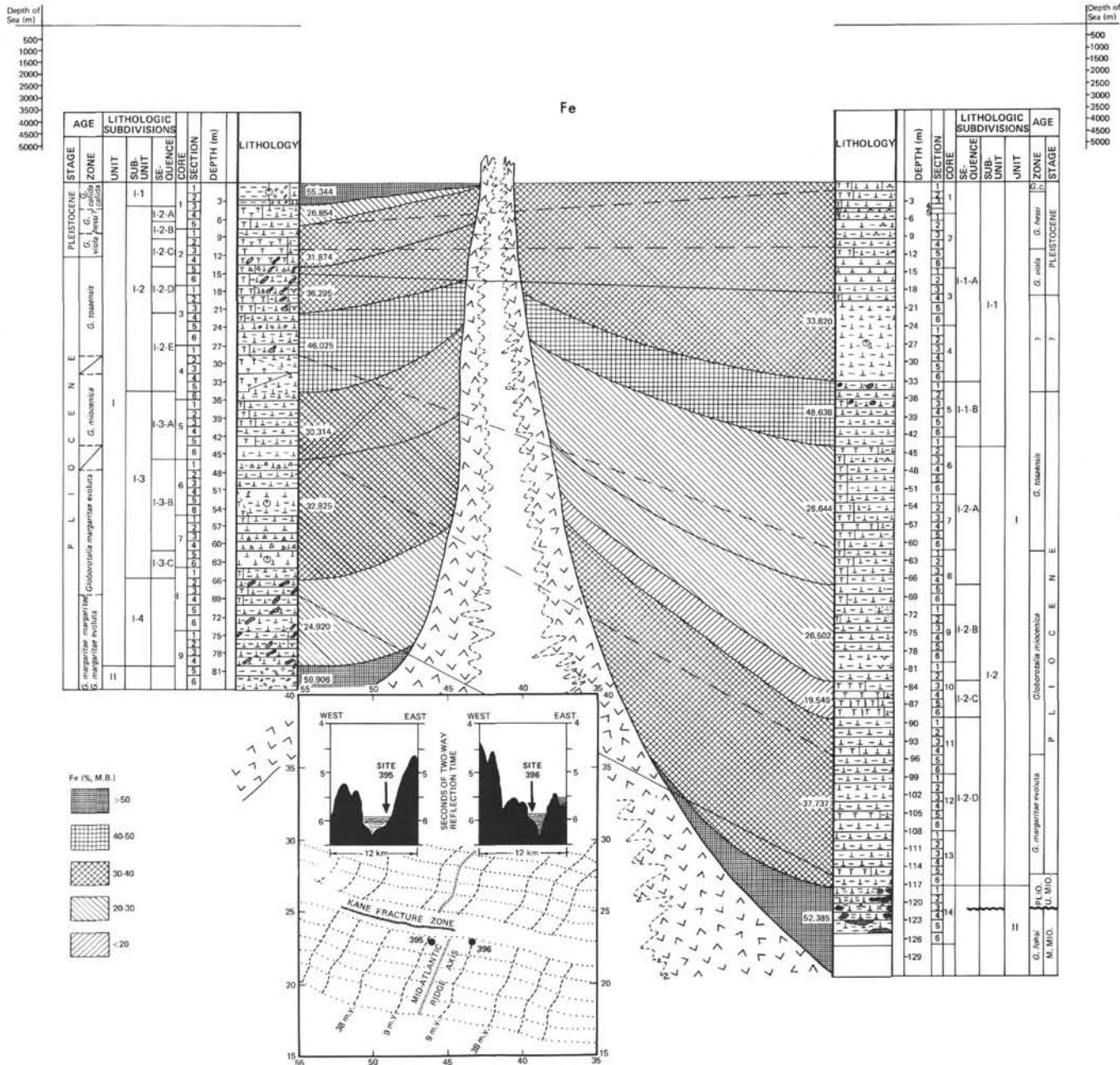
Figure 9. Schematic profile of Fe distribution in upper Cenozoic sediments, region of the Mid-Atlantic Ridge, Leg 45 (wt. %, M.B.).
