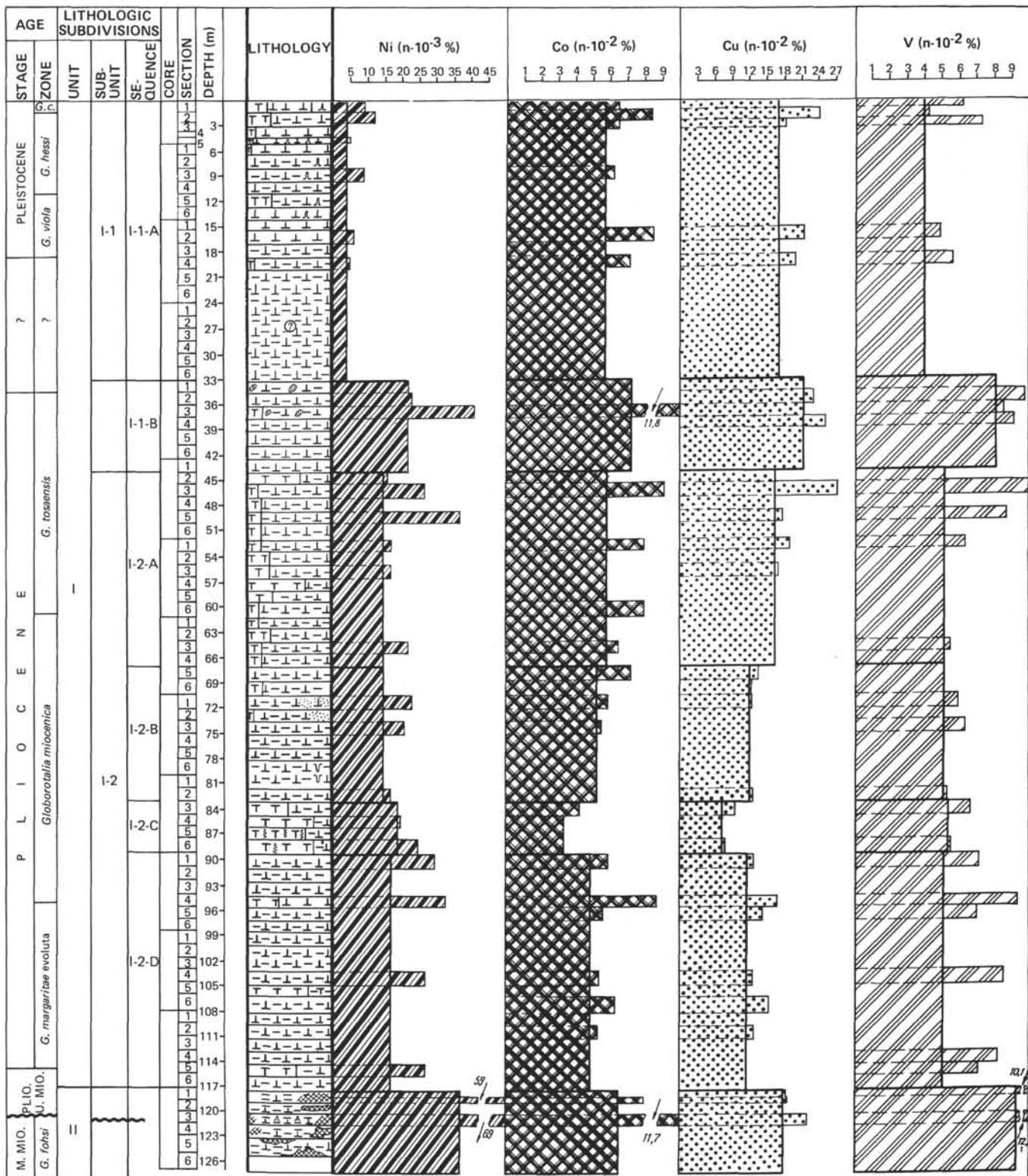
**Figure 5.** Distribution of Ni, Co, Cu, and V (wt. %, recalculated to M.B.) in the section of upper Cenozoic sediments, region of the Mid-Atlantic Ridge, Hole 396, Leg 45.
