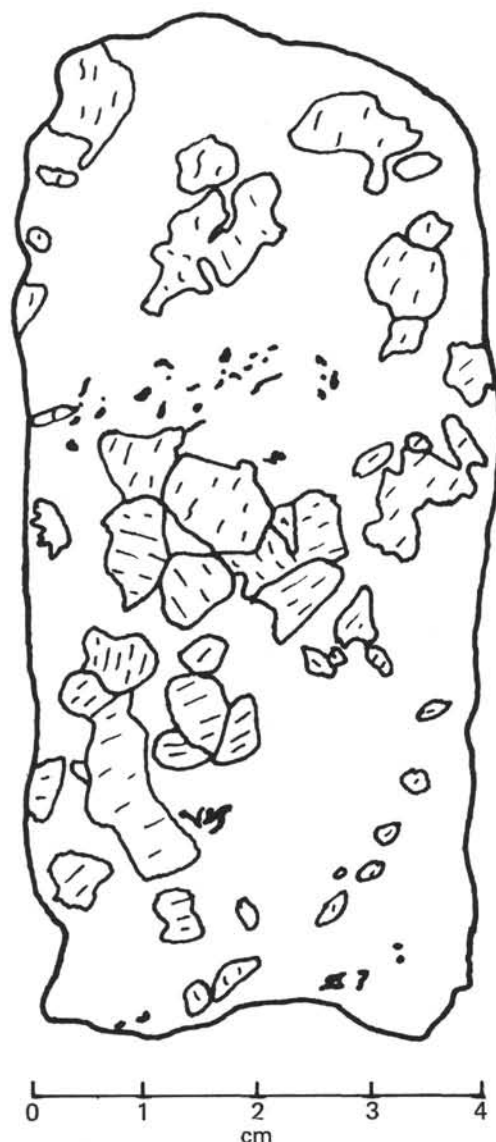
Figure 1. Sketch of a sawed surface of lherzolite Sample 395-18-2, 127-136 cm. Irregular black grains are chrome-spinel; larger cleaved minerals are pyroxenes; unpatterned areas are mainly olivine + serpentine. Note the crude foliation running SW-NE across the figure.
