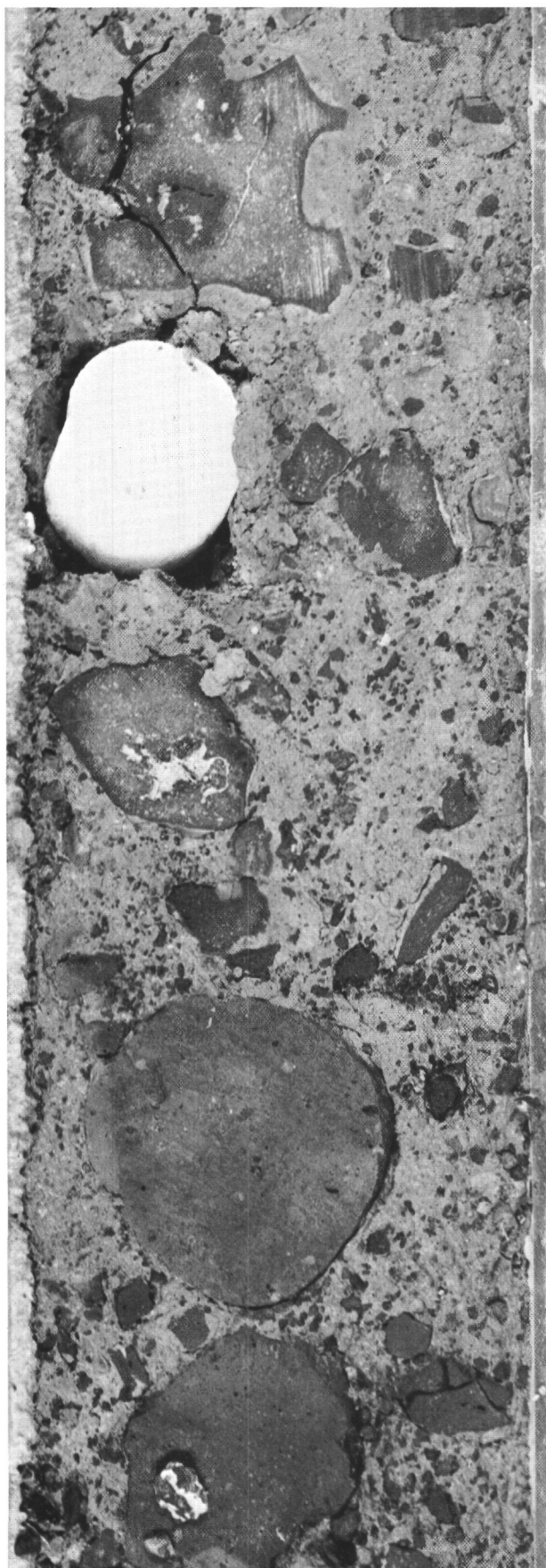
Figure 20. Volcanic breccia with round and angular fragments (Sample 32-1, 40-55 cm).
