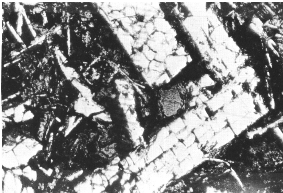
Figure 23. Plagioclase phenocrysts in basalt with tendency to form microcumulate assemblage. One altered olivine phenocryst is evident (322 to 350 m) ( \times 10 ).
