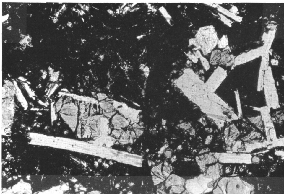
Figure 22. Olivine and plagioclase porphyritic basalt with cryptocrystalline, rather glassy, groundmass (309 to 317 m) (X10).
