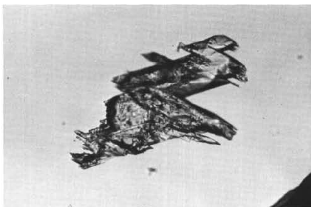
Figure 9. Augite with well-developed hacksaw termination. Sample 445-70-1, 136-137 cm. Greatest length 0.34 mm.
