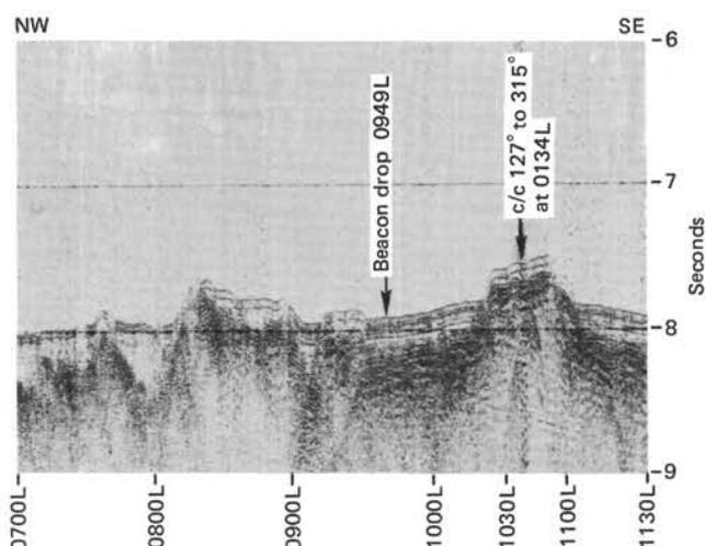
Figure 15. Seismic-reflection profile across Site 447 recorded on board the *Glomar Challenger* during approach to the site.
