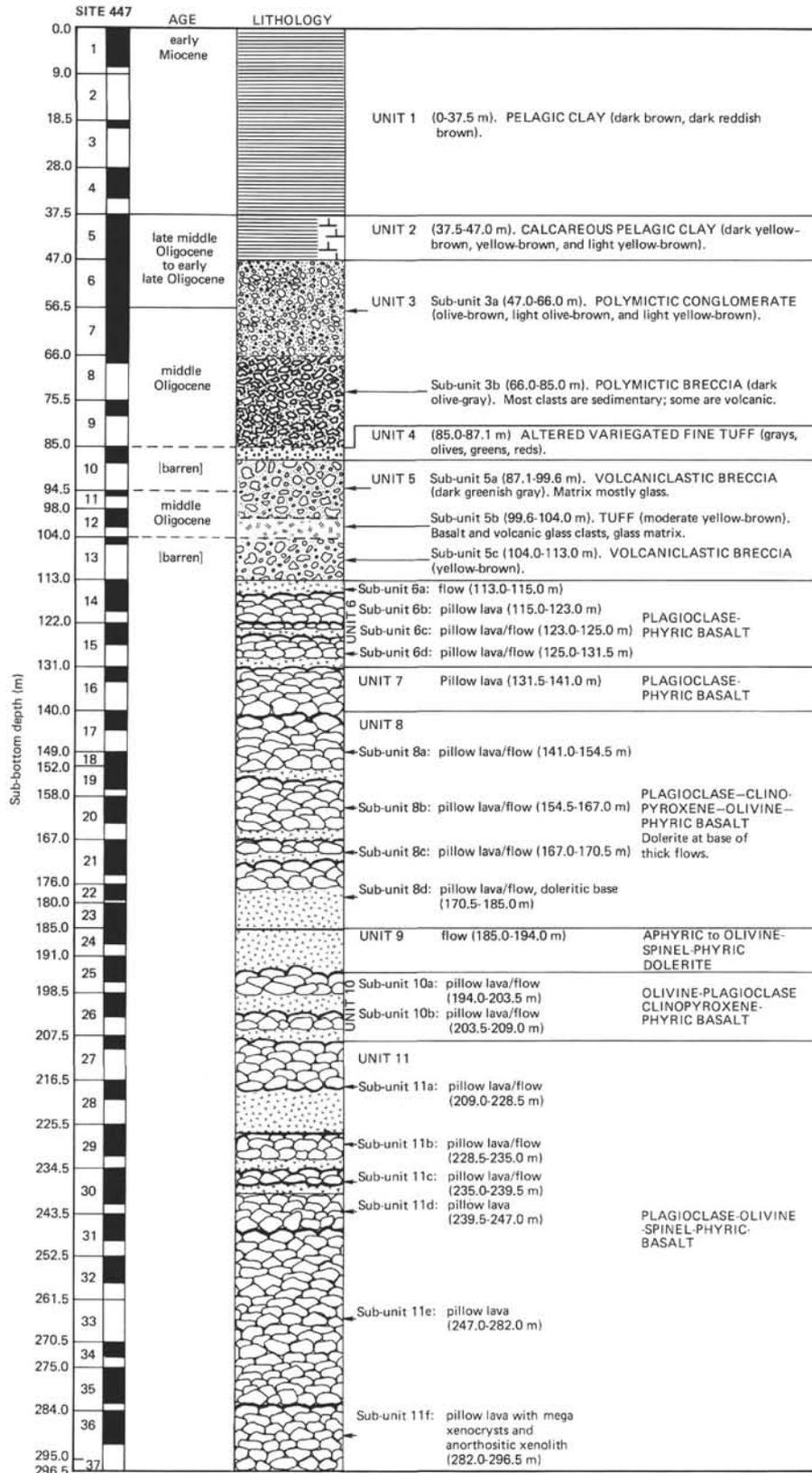
Figure 6. Lithology, age, and core recovery at Site 447. (Heavier lines on pillow tops indicate top of a pillow lava unit or sub-unit. Pillowed massive flows are abbreviated as "pillow lava/flow." Dashed lines in the age column indicate borders of barren intervals. Core recovery is indicated by the solid symbol. Lithologic symbols are summarized in the Introduction [this volume].)
