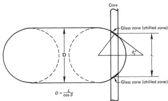
Figure 11. The assumed relative dimensions of pillows. (Estimates of the diameters  $[D]$  of pillows are based upon the measured distance  $[L]$  between the chilled zones in the drill core and the angle  $[\theta]$  formed by the tangent to the chilled zone and the horizontal. The angle  $\theta$  is the measured dip of the glassy margins.)
