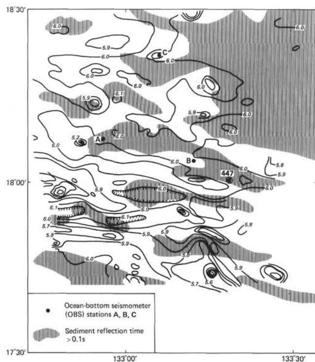
Figure 2. Bathymetry and sediment thickness near Site 447 (L-DGO Site Survey data). (Water depth is contoured in intervals of 0.1 km; shaded sections indicate areas underlain by greater than 0.1 s reflection time of sediment.)
