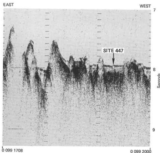
Figure 4. Seismic-reflection profile recorded during preliminary site surveys for Site 447 (L-DGO Site Survey data: *Vema* cruise 34-02, JD 099, 1977; note the profile is from east [left] to west [right]).
