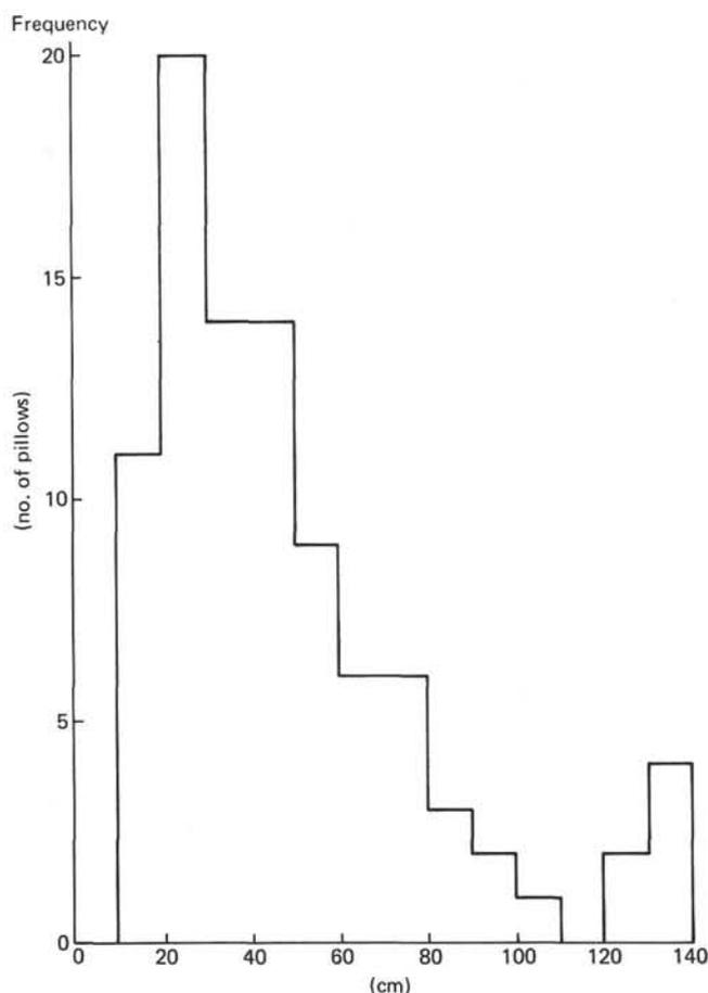
Figure 12. Frequency distribution of the measured minimum diameter of pillows.
