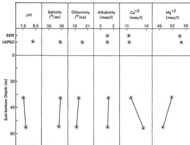
Figure 9. Results of analyses of interstitial water samples versus depth in sub-bottom meters. Values for pH, salinity, chlorinity, alkalinity, and Ca- and Mg-ion concentrations in millimoles per liter are plotted. (IAPSO standard and a surface sea water sample are shown for comparison.)
