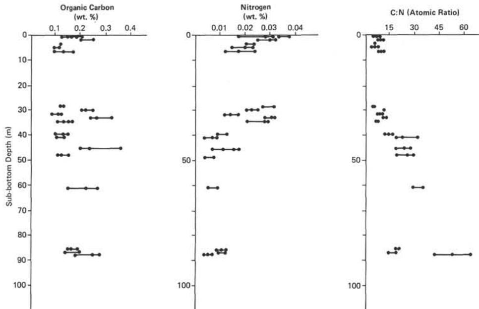
Figure 8. Results of organic carbon and nitrogen analyses of sediment samples versus depth in sub-bottom meters.
