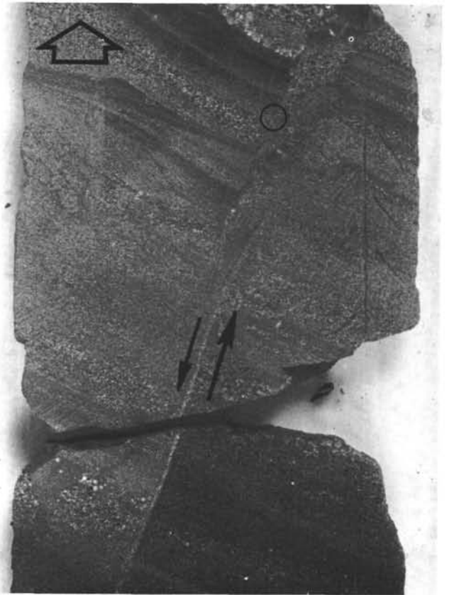
Figure 3. Photograph of a fault zone in carbonate-rich, vitric tuff (Sample 451-42, 385-394.5 m). Outline arrow shows "up" in vertical core. Sense of shear arrows show apparent displacement. Open circle is location of center of thin section shown in Figure 4. Bedding dips \sim 25^\circ to right. Note bifurcation and drag of material above and below open circle along fault. Core diameter is 6.0 cm.
