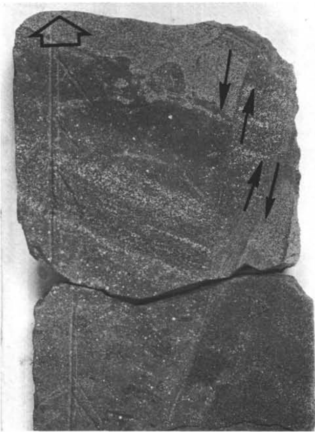
Figure 2. Photograph of a high-angle fault zone developed in carbonate-rich, vitric tuff (Sample 451-42, 335-394.5 m). Fault zone is normal to bedding, which dips 25^\circ to the right. Outline arrow indicates "up" direction in vertical core. Sense of shear arrows reflect apparent displacements. All cores were slabbbed perpendicular to bedding so that the cut surface contains the bedding-dip direction. Accordingly, the narrowness of the fault zone and its steep dip indicate that the strike of the fault is essentially parallel to that of the beds. Core diameter is 6.0 cm.
