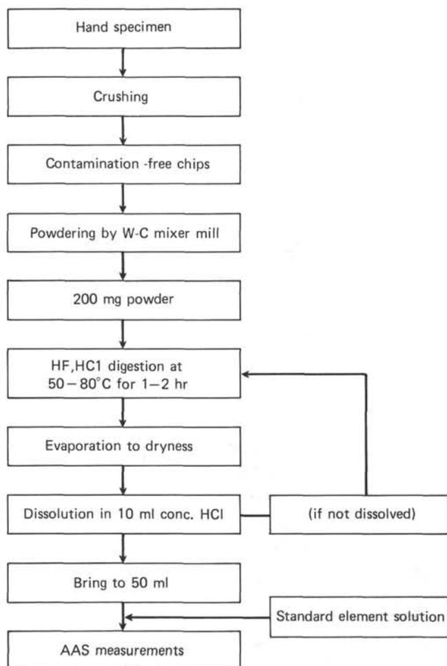
Figure 2. Flow chart of chemical digestion for atomic-absorption spectroscopy.
