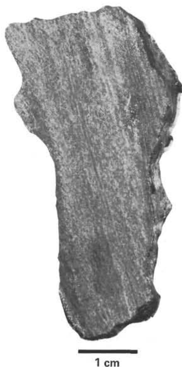
Figure 7. Photograph of 479-13, CC, showing fragment of hard, laminated, dolomitic mudstone.
