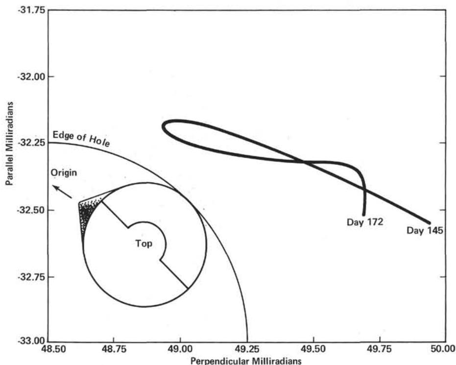
Figure 9. Downhole sensor tilt during the first one-month deployment. (Each point on the curve represents one hour. On the basis of the seismic arrival characteristics, the sensor package orientation is estimated to be north-south in the parallel tilt direction and east-west in the perpendicular tilt position. Thus the tilt motion is mainly in a direction along the strike of the trench.)
