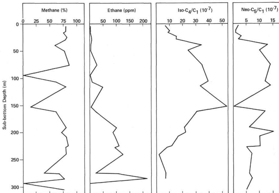
Figure 13. Concentrations of gaseous hydrocarbons at Site 494.
