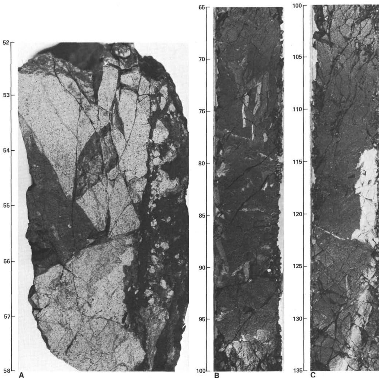
Figure 3. Deformation fabric of dark gray Eocene mudstones. (Off-sets, conjugate fractures, and healed fractures are outlined by light colored bands rich in volcanic glass.) A. Sample 494A-27-3, 52–58 cm; B. Sample 494A-27-1, 65–100 cm; C. Sample 494A-27-1, 100–135 cm.
