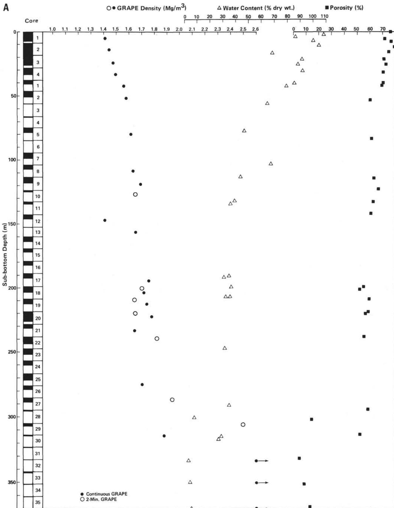
Figure 4. A and B. Physical properties of the lithologic section at Site 494. (A. Arrows denote points outside the range of the graph for GRAPE density data.)
