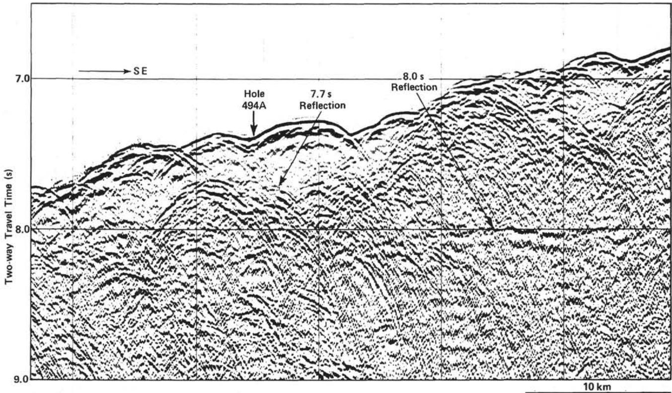
Figure 7. Portion of a multichannel record (GUA-9) perpendicular to and crossing GUA-18 at Site 494, which shows reflections beneath the seaward extremity of the Guatemalan margin. (The reflection at 7.7 s occurs 0.4 s below the seafloor.)
