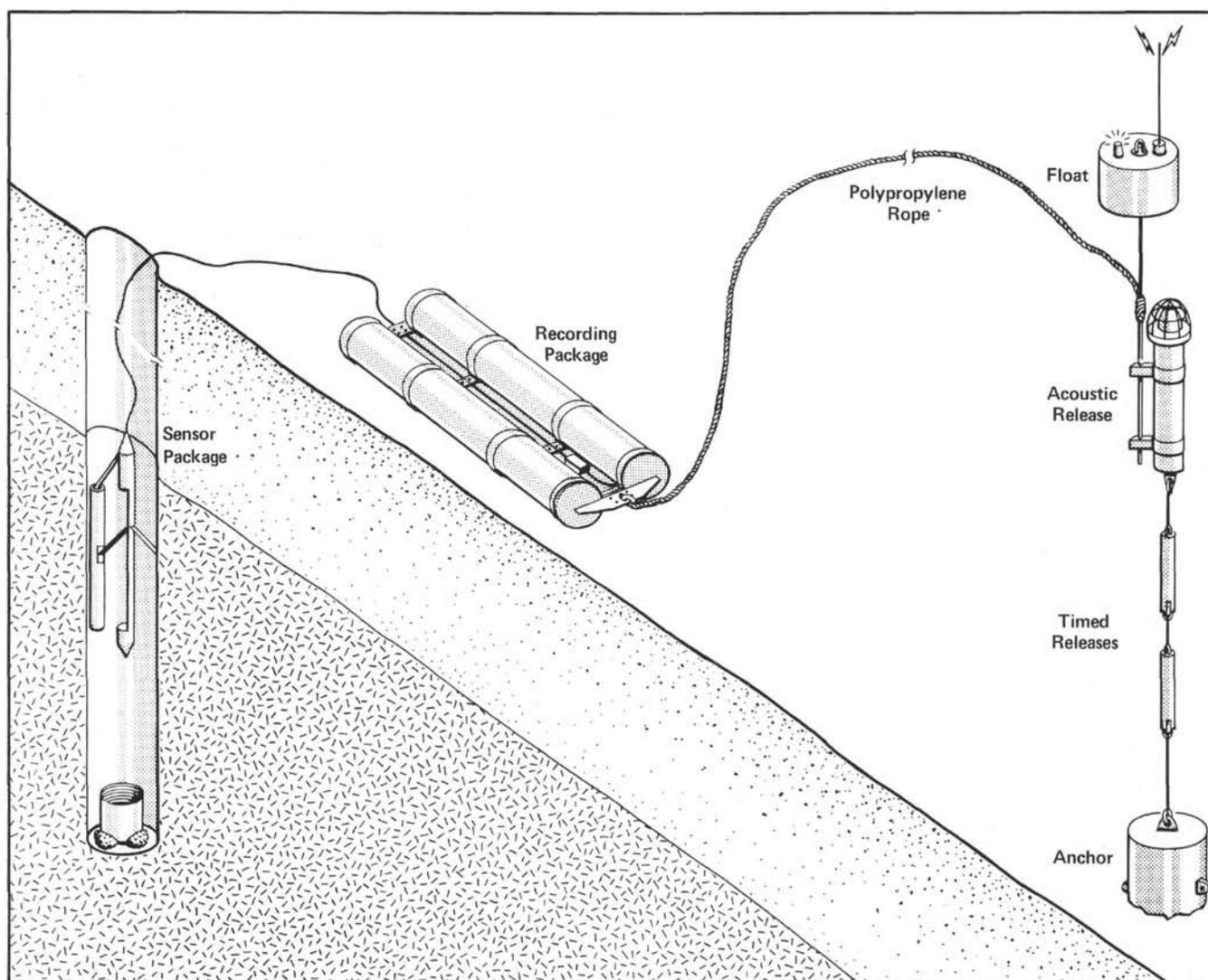
Figure 8. The ocean-sub-bottom seismometer system as deployed in DSDP Hole 494A. (The length of the logging cable from the sensor package downhole to the recording package on the seafloor is more or less 9100 m; an additional 9000 m of 1 1/4-in. polypropylene rope separates the recording package from the recovery float, which will bring the end of the rope to the ocean surface after activation of any of the releases.)
