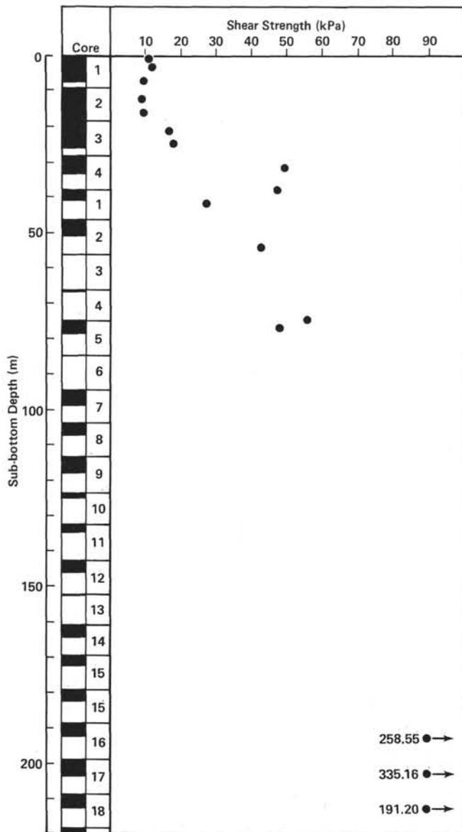
Figure 5. Shear strength of sediment from Site 494. (Arrows denote points outside the range of the graph.)
