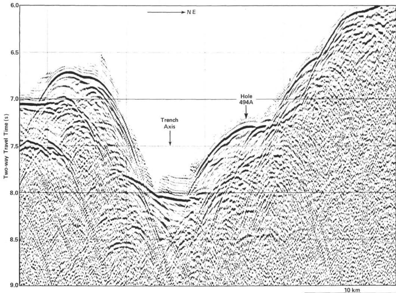
Figure 6. A 10 to 50 Hz seismic-reflection record (GUA-18) representative of the records collected during the UTMSI site survey of the Guatemalan margin.
