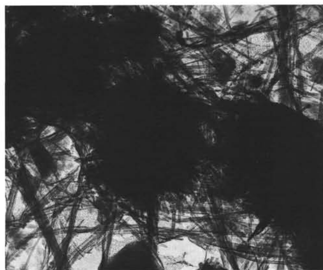
Plate 1. Electronmicrographs. 1. Sample 530B-22-3, 71 cm ( \times 8,000 ); early Pleistocene; well-shaped particles of illite, fleecy particles of smectite, and fragments of diatoms. 2. Sample 530A-39-2, 83 cm ( \times 12,500 ); early Eocene; palygorskite in long and straight fibers, smectite with blurred contours, and well-shaped illite. 3. Sample 530A-39-2, 83 cm ( \times 20,000 ); early Eocene; Palygorskite in long and straight fibers, smectite with blurred contours, and well-shaped illite. (Some fibers appear to grow at the periphery of dense particles.) 4. Sample 530A-39-2, 83 cm ( \times 40,000 ); early Eocene; Fibers of palygorskite growing at the periphery of dense particles (detail of Fig. 3).
