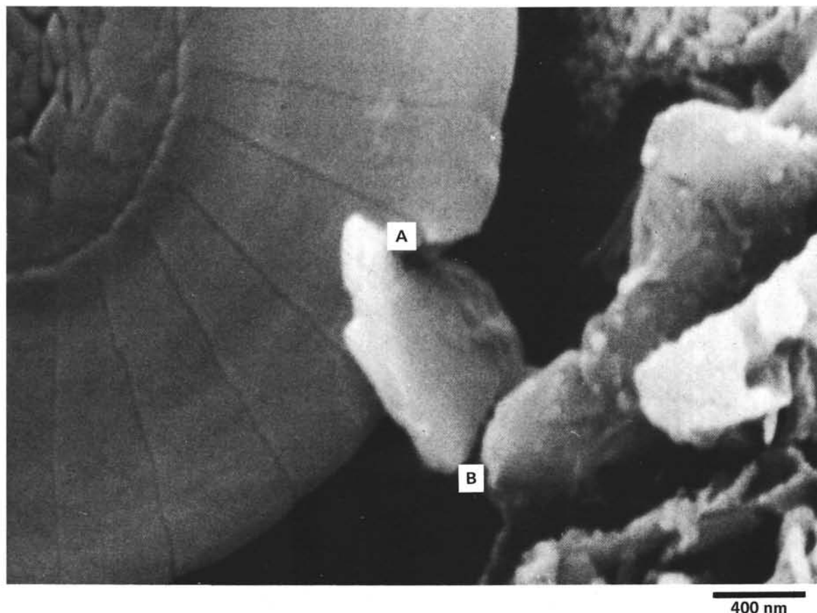
Figure 4. SEM photomicrograph (Section 12-3) illustrating structure stabilizing effect of carbonate: (A) solution feature at a coccolith and (B) carbonate precipitation stabilizing the sediment.
