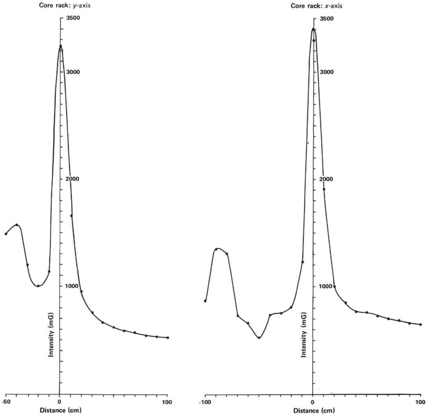
Figure 7. The total field intensity measured at 10-cm intervals in the horizontal  $x$  and  $y$  directions near the core rack. The intensity in the vertical direction was too high to be measured on the magnetometer in the  $z$  and  $y$  directions, thus no  $z$  axis measurements are shown.
