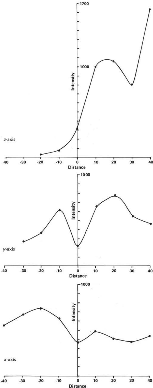
Figure 4. Profile of the total magnetic field intensity associated with the top of the drill string. The horizontal direction is parallel to the length of the *Glomar Challenger*. The positive  $y$  direction is in the direction of the bow. The vertical field was measured from a height of 40 cm above the collar to a depth of 20 cm within the collar.
