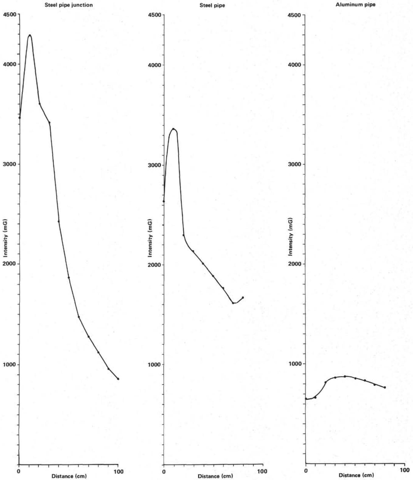
Figure 6. Total field intensity associated with drill pipes. These surveys were limited to the horizontal direction perpendicular to the pipe rack.
