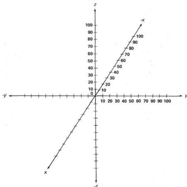
Figure 1. Illustration of orthogonal framework for measurements. The two horizontal axes are  $90^\circ$  apart with the vertical ( $z$  axis)  $90^\circ$  from the  $x$  and  $y$  orthogonal axis. Measurements were made in 10-cm intervals along each axis.
