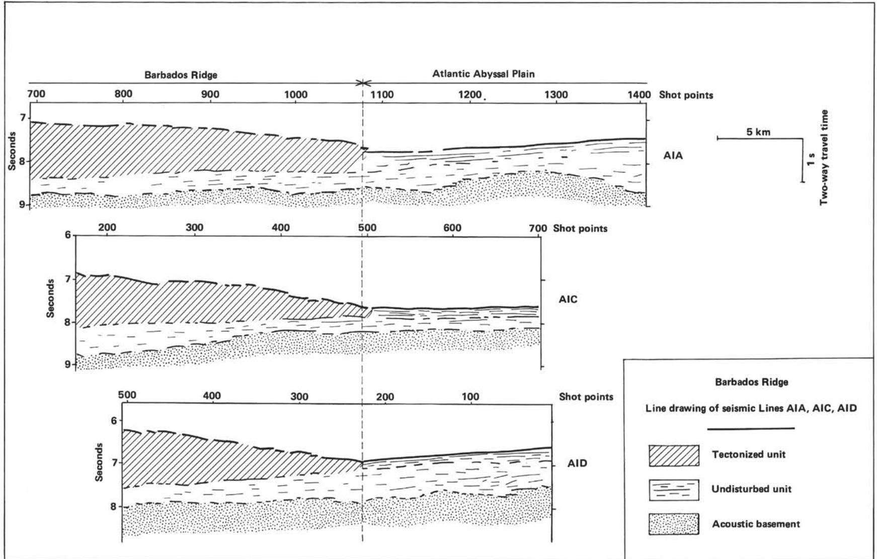
Figure 8. Interpreted sections of Lines A1A, A1C, and A1D through the deformation front showing the continuity of the seismic units from north to south of the survey and local thickness variations.
