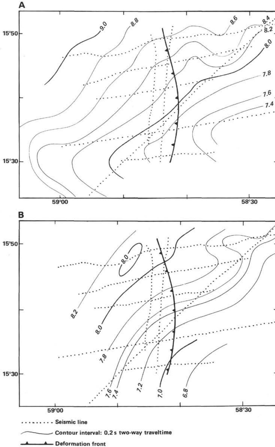
Figure 11. A. Isotime map of the basement showing the northwest deepening of the basement oblique to the deformation front and the seafloor topography. B. Isotime map of Reflector 1; note the northwest deepening of Reflector 1 oblique to the deformation front. Contours are given in seconds of two-way traveltime.
