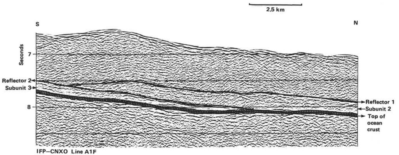
Figure 14. Example of thickness variation of Subunits 2 and 3 on Line A1F. Subunit 3 thins northward due to the basement topography (it may be very thin on the high but is not resolved by conventional seismic means). Subunit 2 thins to the south along a surface interpreted as a tectonic truncation. If true, this interpretation would mean that at least locally the décollement is not along a stratigraphic level and that Subunit 2 is scraped off too.
