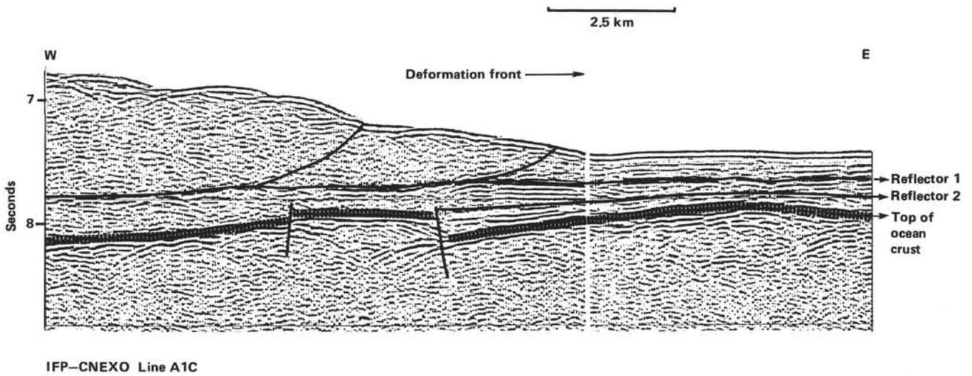
Figure 13. Faulted basement highs on Line A1C below the toe of Barbados Ridge. Note the thickness variation of Subunit 3 below Reflector 2.
