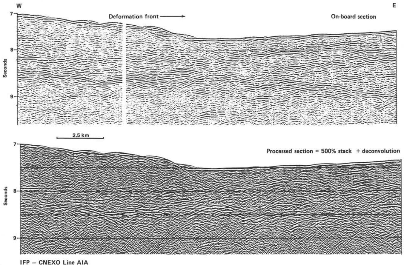
Figure 5. Comparison between on-board and processed sections.
