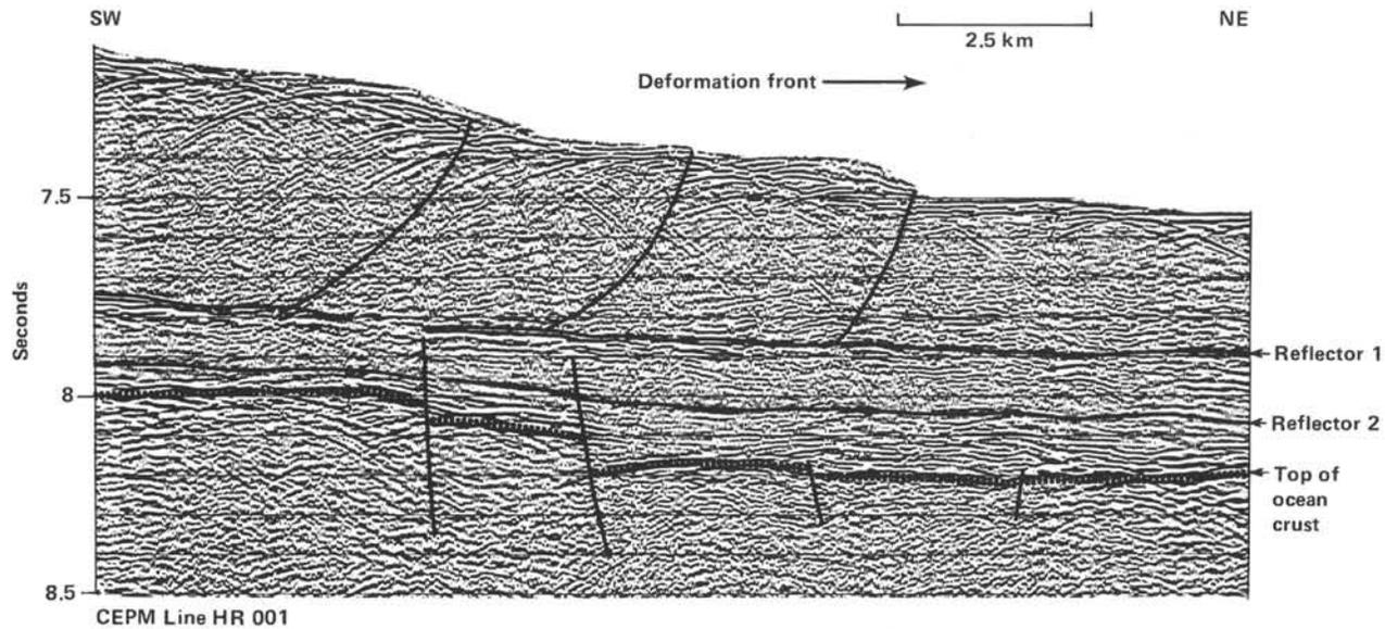
Figure 6. High resolution CEPM multichannel seismic line HR 001. Better resolution is achieved than in Figure 5. Nevertheless the internal structure of the upper unit (above Reflector 1) is badly understood. Drawing of the reverse fault is highly speculative before drilling information is obtained. This profile allows the definition of Reflector 2 into the layered sequence.
