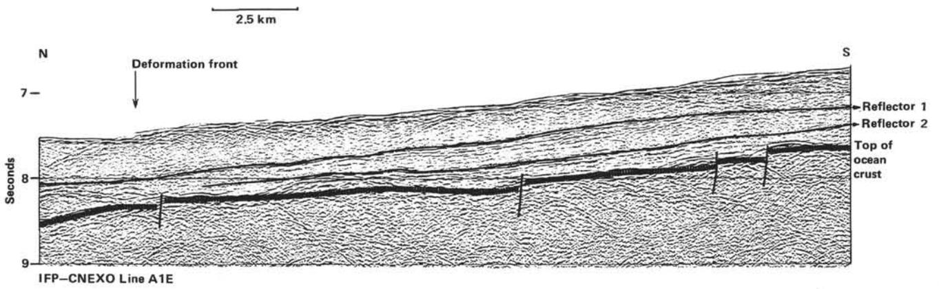
Figure 12. Northward deepening of the basement on Profile A1E. Over 50 km from south to north, the top of ocean crust deepens about 1 s (1000 m).
