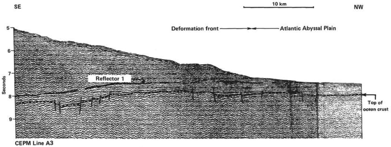
Figure 3. Main structural sequences at the deformation front. Below the lower slope between the seafloor and Reflector 1, there is an acoustically discontinuously reflective subunit interpreted as a pile of deformed sediments. Between Reflector 1 and the top of the ocean crust there is a well-layered sequence of reflectors interpreted as an autochthonous tegument above the ocean crust. A very diffracting acoustic basement is interpreted as the ocean crust.
