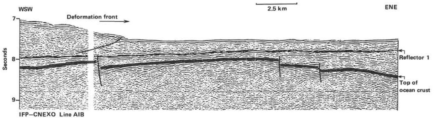
Figure 10. Example of the faulted ocean basement and correlative thickening of the infra-Reflector 1 sequence.
