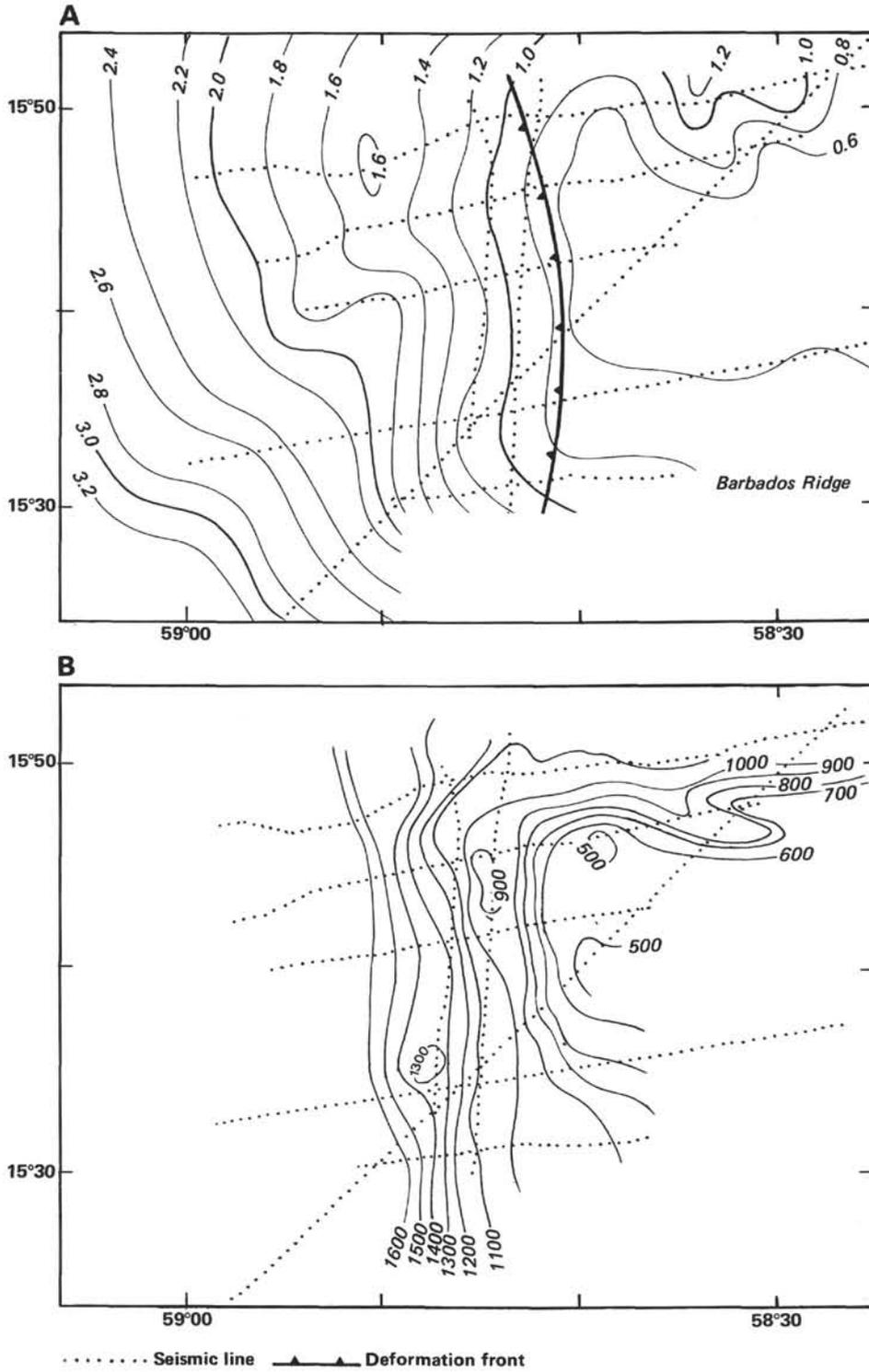
Figure 9. Total sediment thickness A. in time(s) and B. converted in meters.
