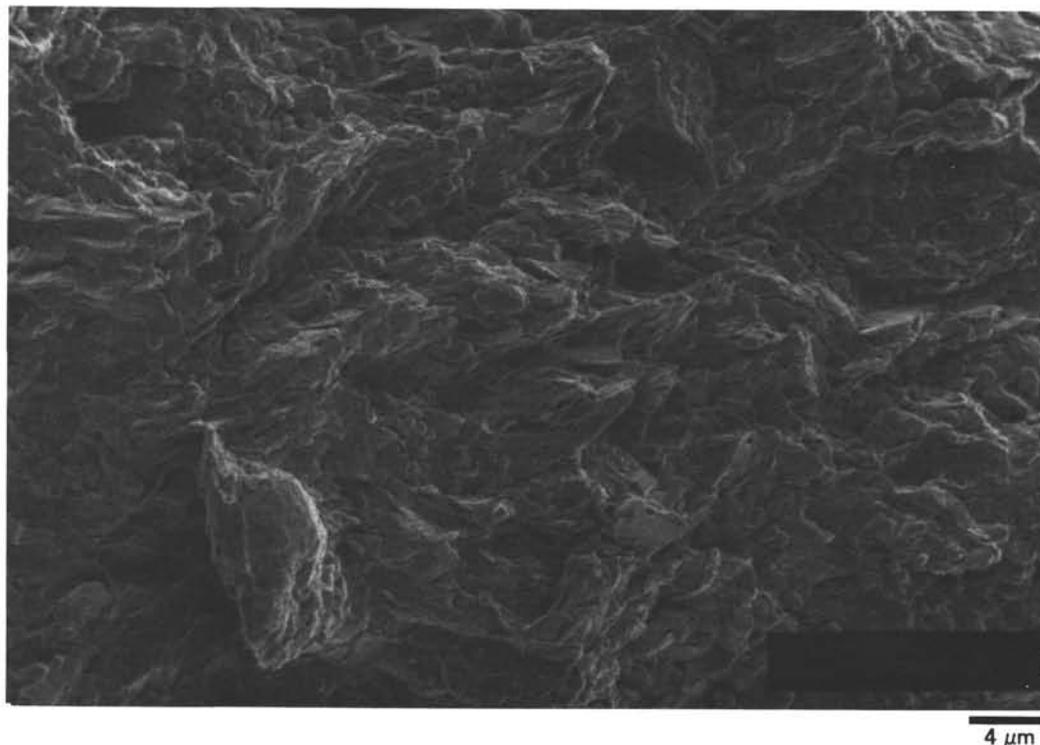
Figure 11. SEM photomicrograph of clay-rich lower Miocene radiolarian mud from décollement zone—Sample 541-50-3, 51-55 cm. (Photomicrograph illustrates moderate preferred orientation of platy minerals due to penetrative microscopic slip.)
