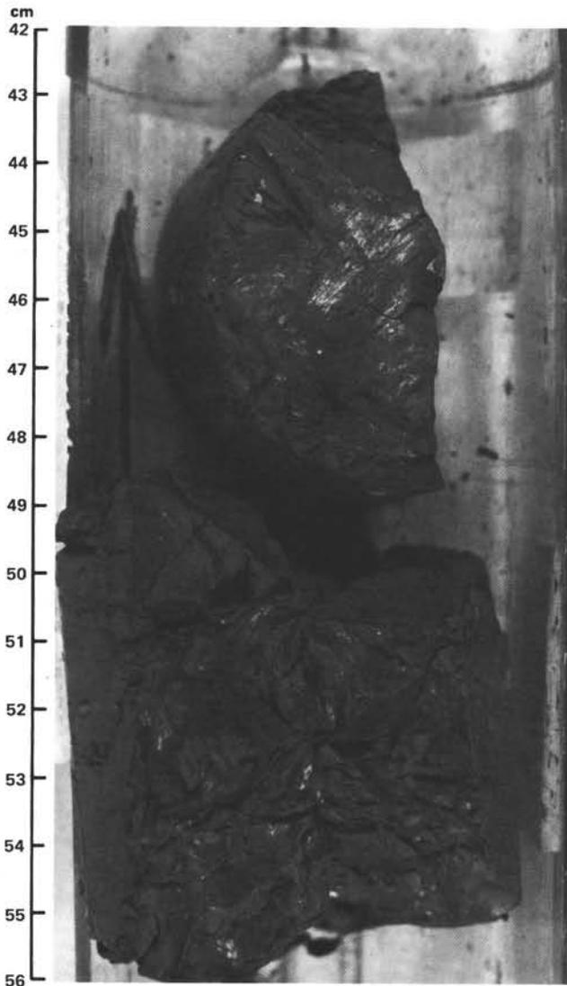
Figure 4. Photograph of the interior of the core-catcher from Site 541, Core 25. (Diversely oriented, polished and striated, mesoscopic slip surfaces are distributed throughout the mud.)
