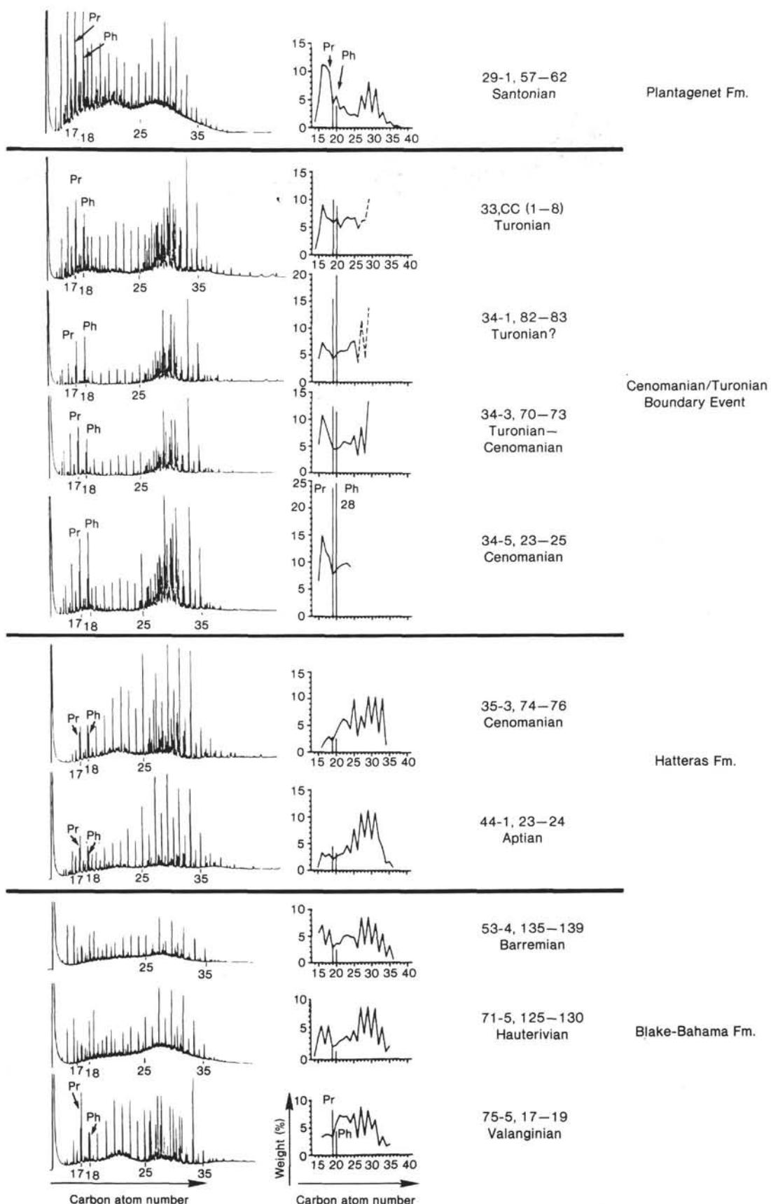
Figure 4. Chromatogram of the saturated + unsaturated fraction of samples from Hole 603B, Gas chromatography analysis on quartz col. capil. CP SIL5 ( $\theta$  int: 0.5 mm, L = 25 m), injected 0.2  $\mu$ l splitless (model Varian 3700). Pr = pristane, Ph = phytane.
