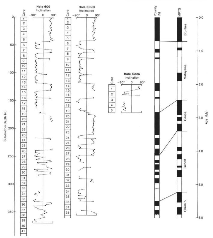
Figure 8. Results for Site 609 samples after treatment at 10 mT. See Figure 4 caption for further explanation.
