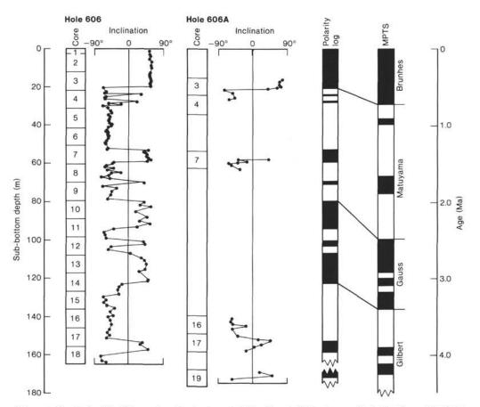
Figure 4. Results for Site 606 samples after treatment at 10-mT peak field, shown with inclinations plotted versus sub-bottom depth. The depths of the tops of the cores are indicated. The inclination records are summarized in a composite polarity log for Site 606. The composite log is correlated with the magnetic polarity time scale (MPTS). The time scale is plotted relative to the ages shown at the right side of the figure. See Appendix for specific depths of reversals.
