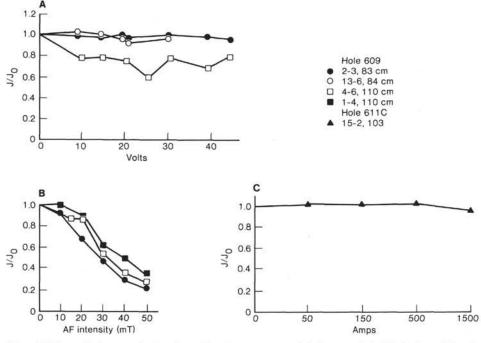
Figure 2. Normalized magnetization intensities after treatment with the osmotic knife. A. Intensities after treatment at progressively higher voltages. B. Intensities during progressive AF demagnetization of two samples which had been treated at 49 V with the knife and, for comparison, one untreated sample (609-1-4, 110 cm). C. Intensities after treatment at progressively higher amperages.
