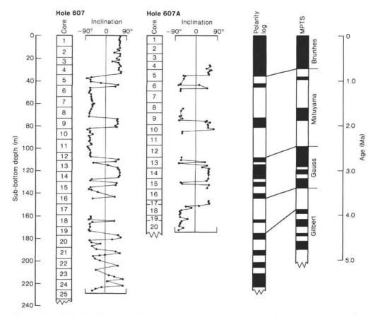
Figure 5. Results for Site 607 samples after treatment at 10 mT. See Figure 4 caption for further explanation.
