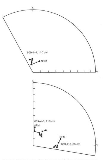
Figure 1. Magnetization directions measured after treatment at progressively higher voltages using the osmotic knife, plotted on equalarea projections.
