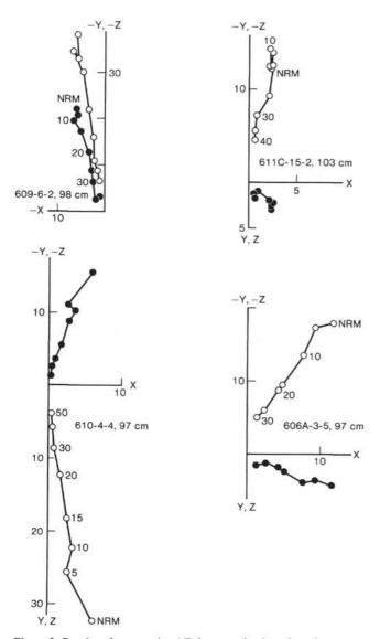
Figure 3. Results of progressive AF demagnetization plotted as vector endpoint diagrams (Zijderveld, 1967). Open symbols represent projections onto the vertical plane; solid symbols represent projections onto the horizontal plane. AF intensity in milliteslas; magnetization intensity in units of  $10^{-3}$  A/m.
