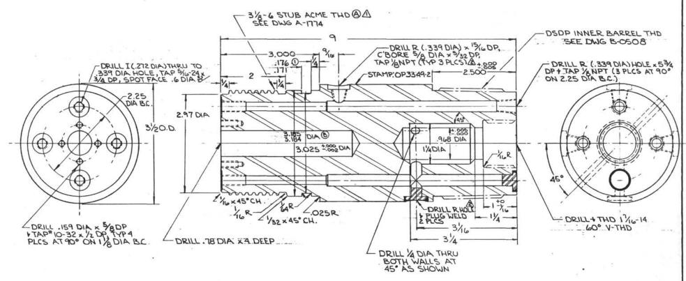
NOTE: DIA A+ B TO BE CONCENTRIC WITHIN .0005 FULL INDICATOR READING.
