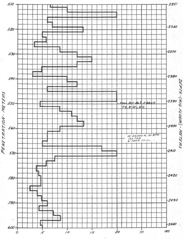
CORING & DRILLING RATE - METERS / HOUR
