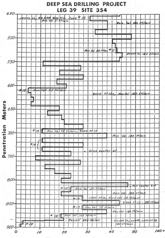
Drilling & Coring Rate motors /hour
