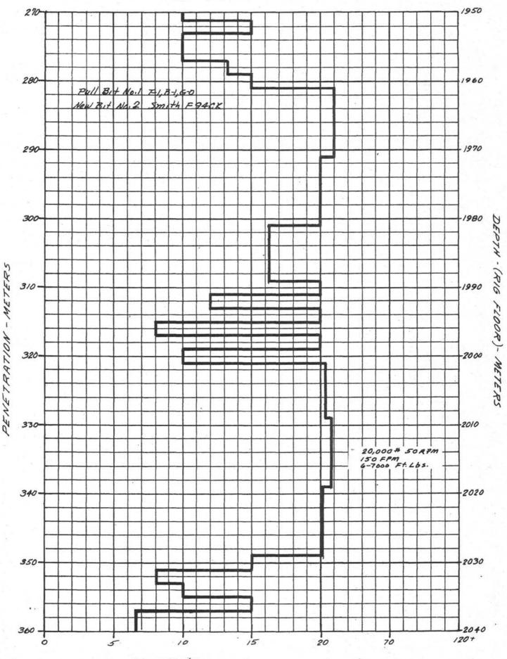
CORING & DRILLING RATE METERS HOUR
