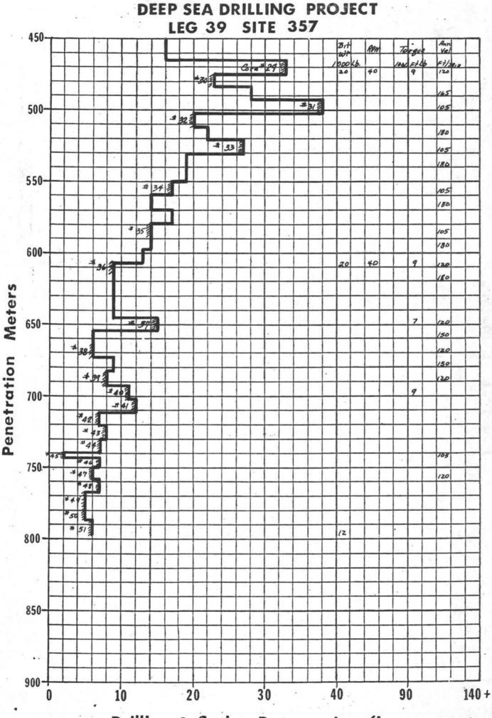
Drilling & Coring Pate meters/hour
