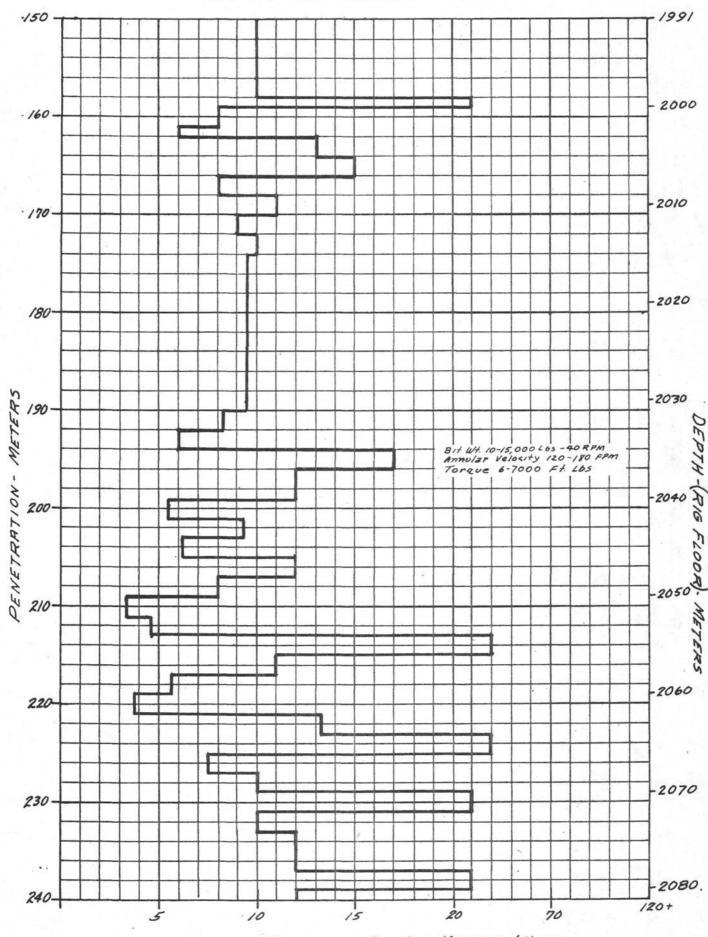
CORING & DRILLING RATE - METERS / HOUR
